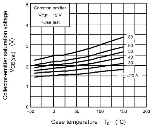
**Fig. 8.5  $V_{CE(sat)} - T_c$**
