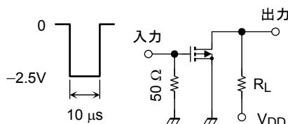
$V_{DD} = -3\text{ V}$
