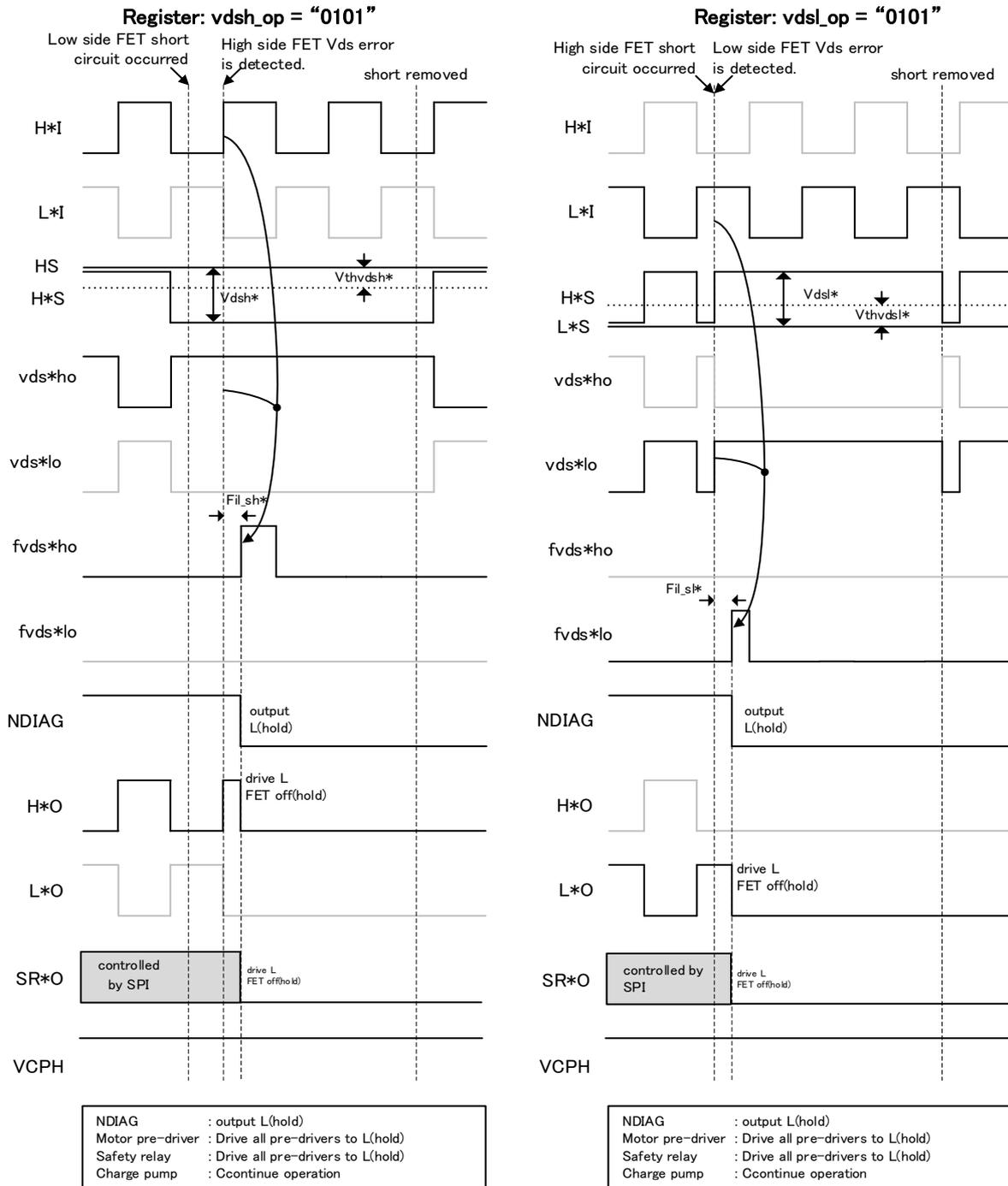
Fig. 7.5.8-g Timing chart for short-circuit detection (register vds\_l\_op = vds\_h\_op "0101")
