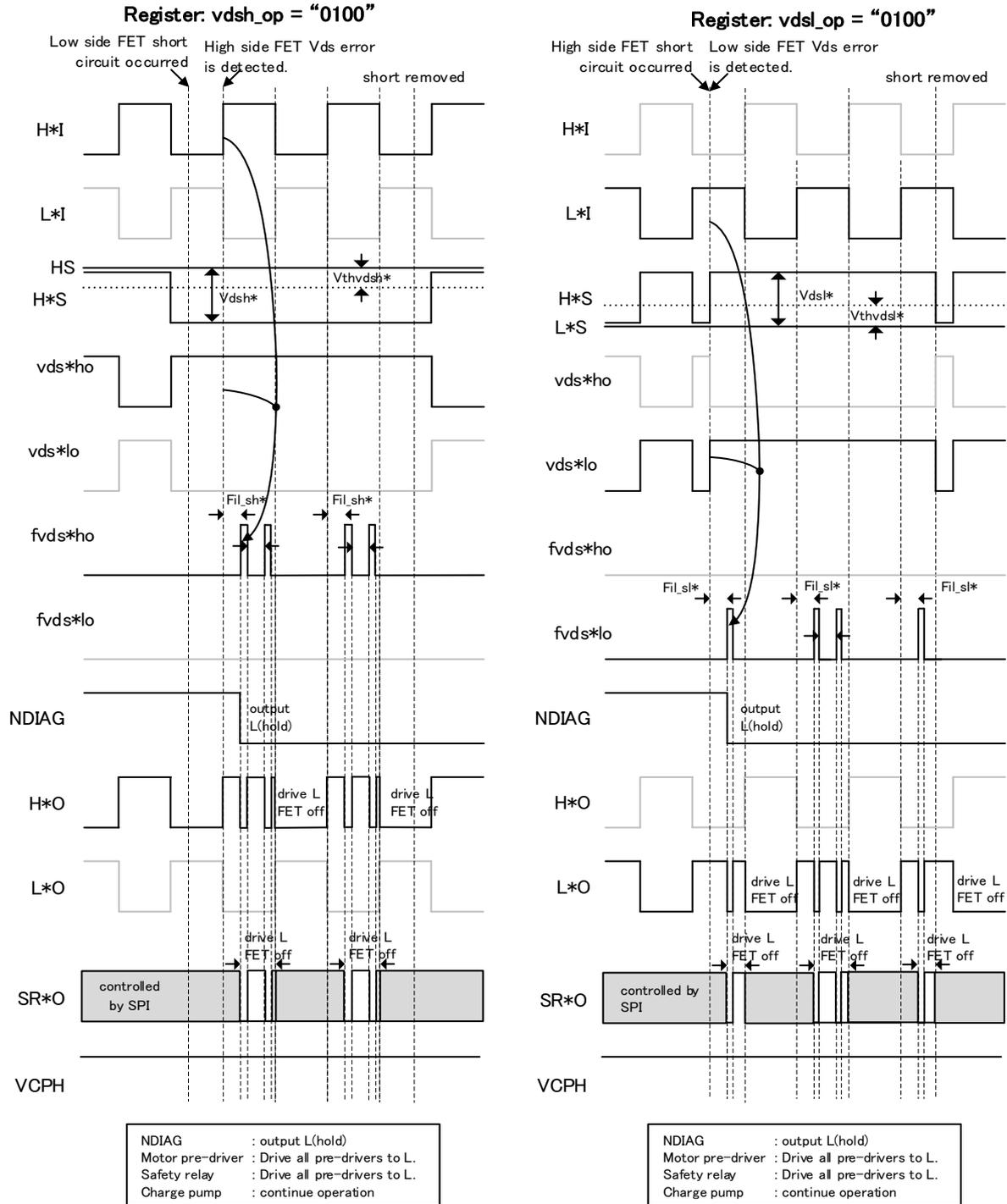
Fig. 7.5.8-f Timing chart for short-circuit detection (register vds<sub>l</sub>\_op = vds<sub>h</sub>\_op "0100")
