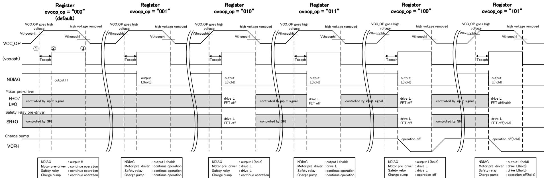
Fig. 7.5.6-b Timing chart for VCC\_OP overvoltage detection
