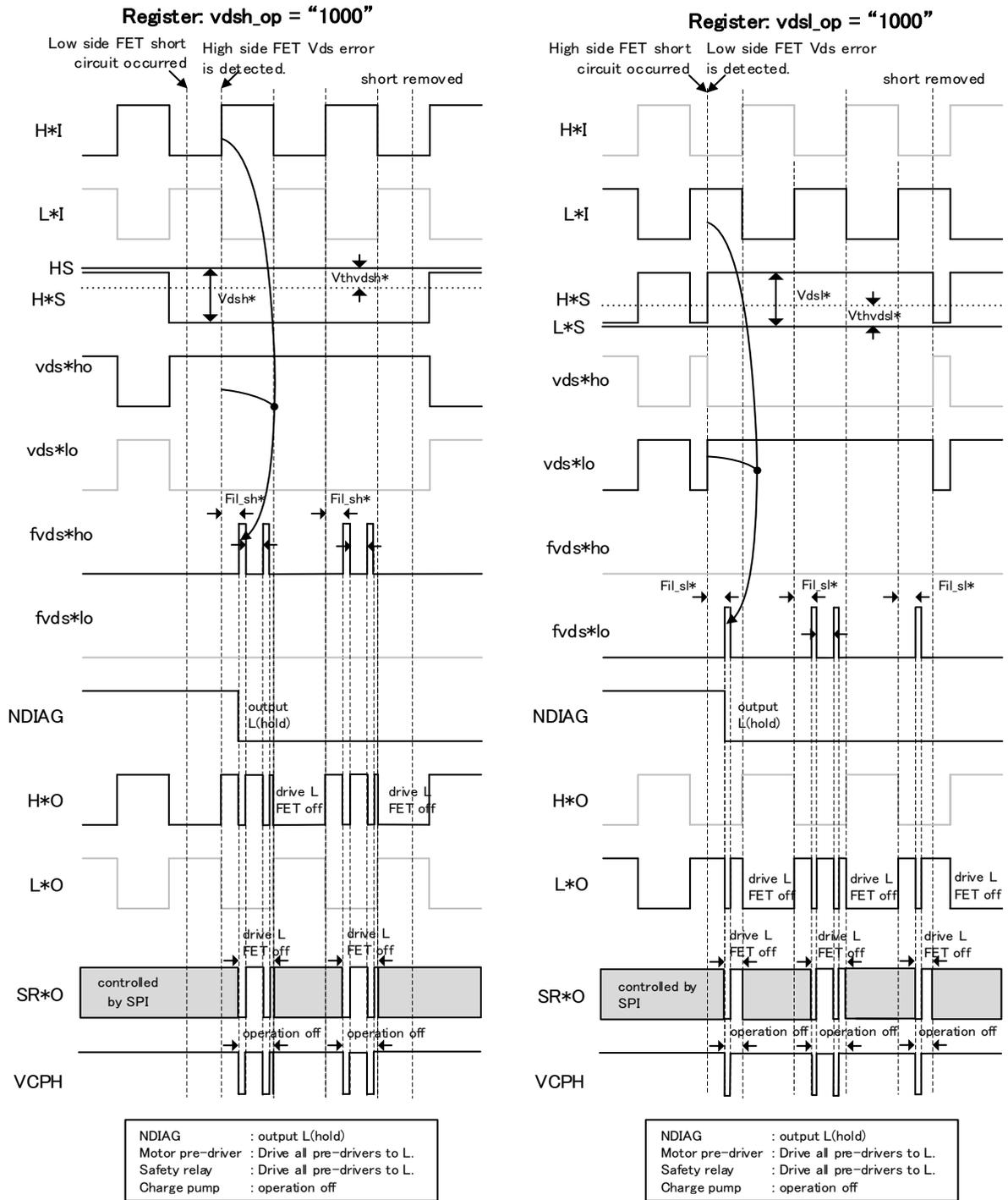
Fig. 7.5.8-j Timing chart for short-circuit detection (register vdsi\_op = vds\_op "1000")
