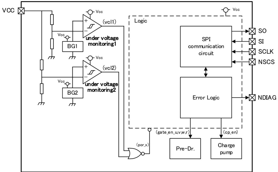
**Fig. 7.5.1-a Block diagram for VCC undervoltage detector**
