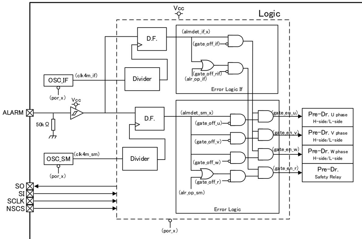
Fig. 7.6-a MOSFET drive circuit control block diagram
