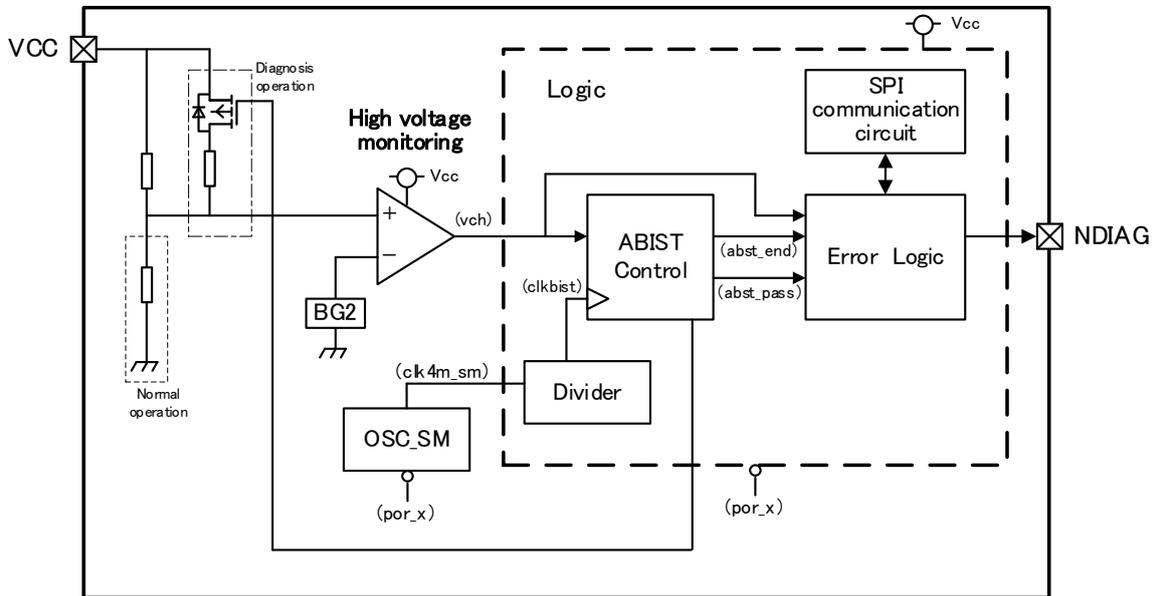
**Fig. 7.7-a ABIST block diagram (VCC overvoltage detection)**
