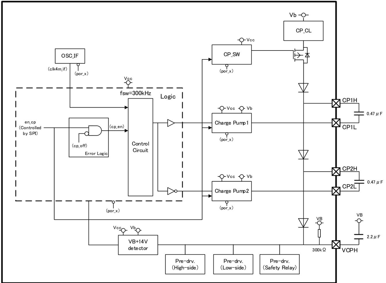
Fig. 7.1-a Block diagram for charge pump circuit
