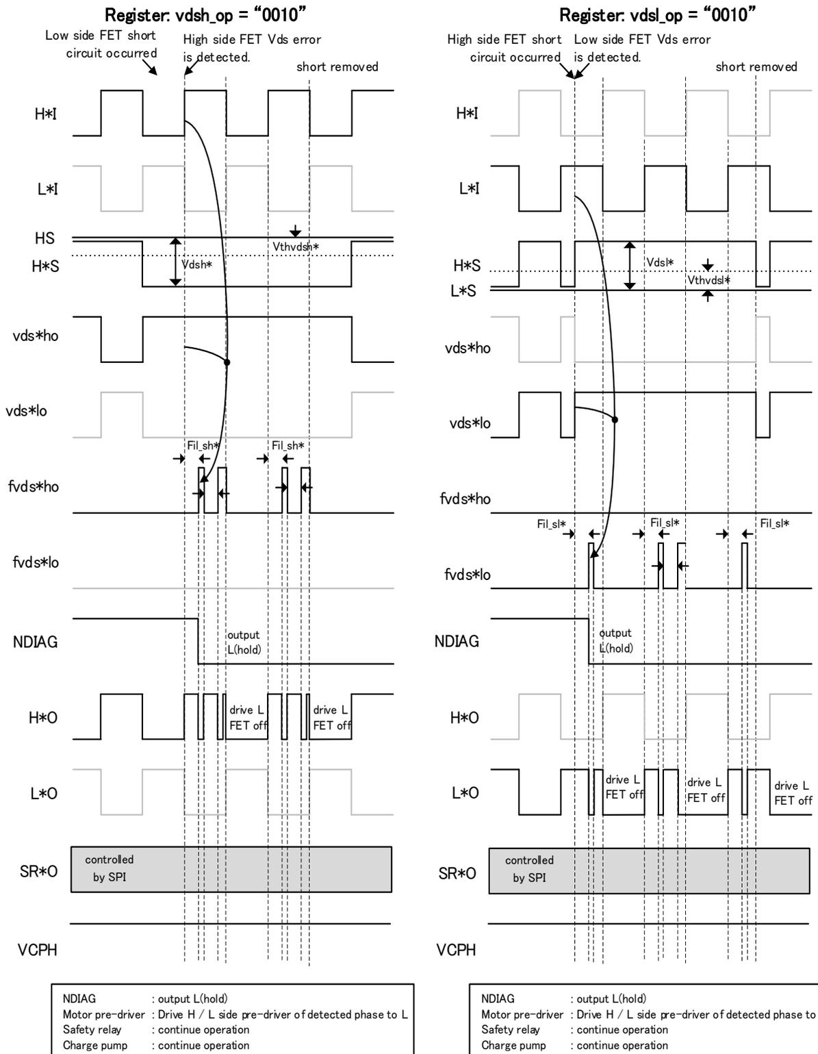
**Fig. 7.5.8-d Timing chart for short-circuit detection (register vds<sub>l</sub>\_op = vds<sub>h</sub>\_op "0010")**
