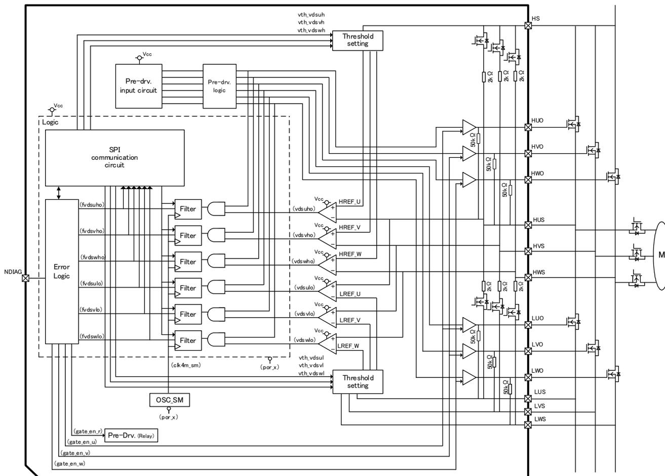
Fig. 7.5.8-a Block diagram for external MOSFET VDS detection
