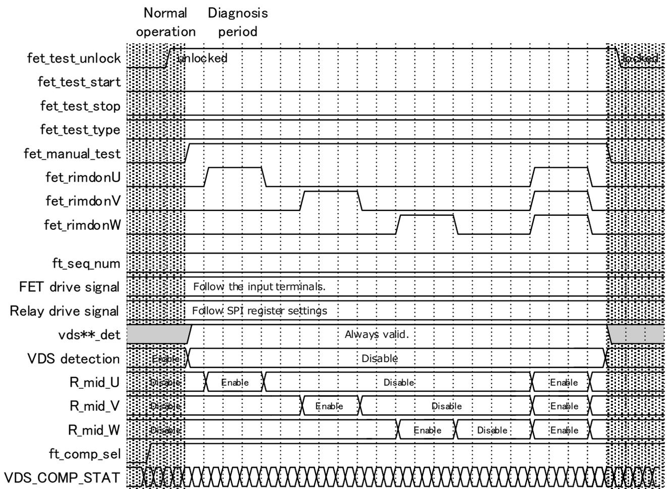
Fig. 7.8-b Operation waveforms in the manual inspection mode
