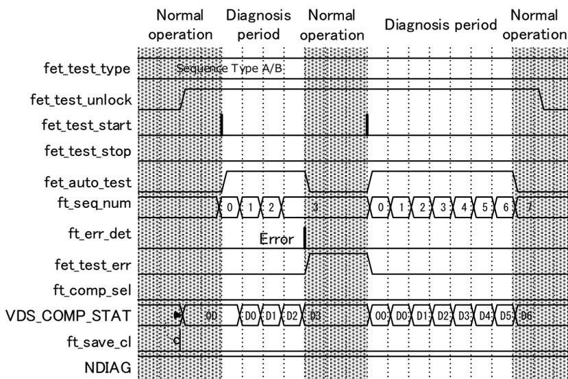
Fig. 7.8-h Operation waveforms when expectation disagreement is detected
