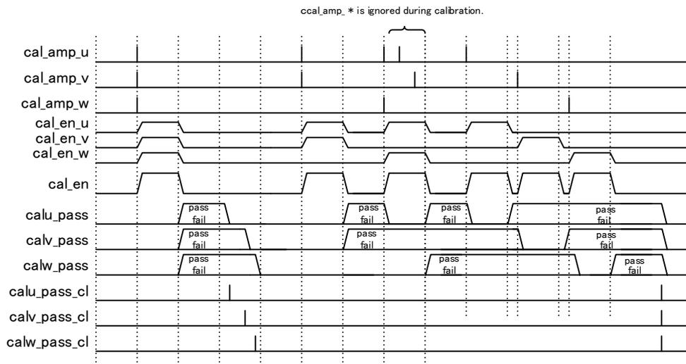
Fig. 7.3-d Offset calibration
