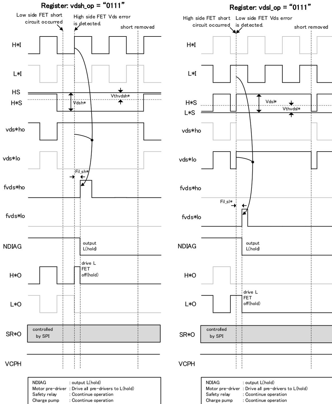
Fig. 7.5.8-i Timing chart for short-circuit detection (register vds<sub>l</sub>\_op = vds<sub>h</sub>\_op "0111")
