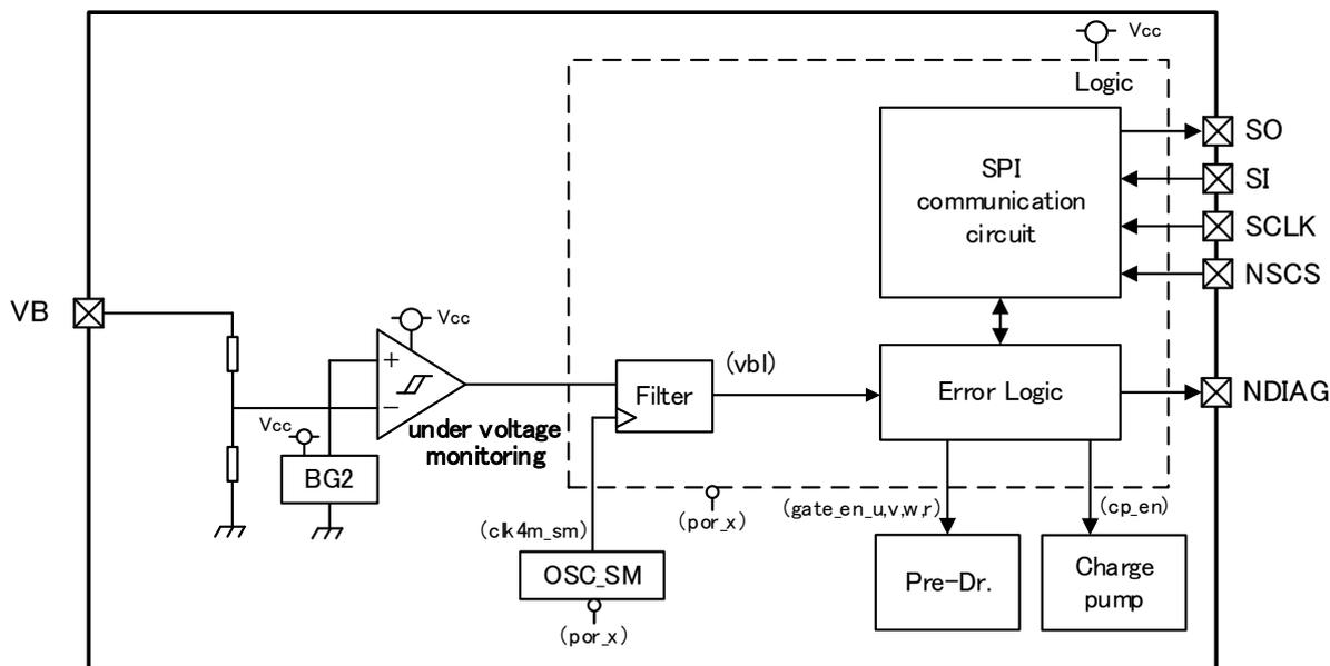
Fig. 7.5.2-a Block diagram for VB undervoltage detection
