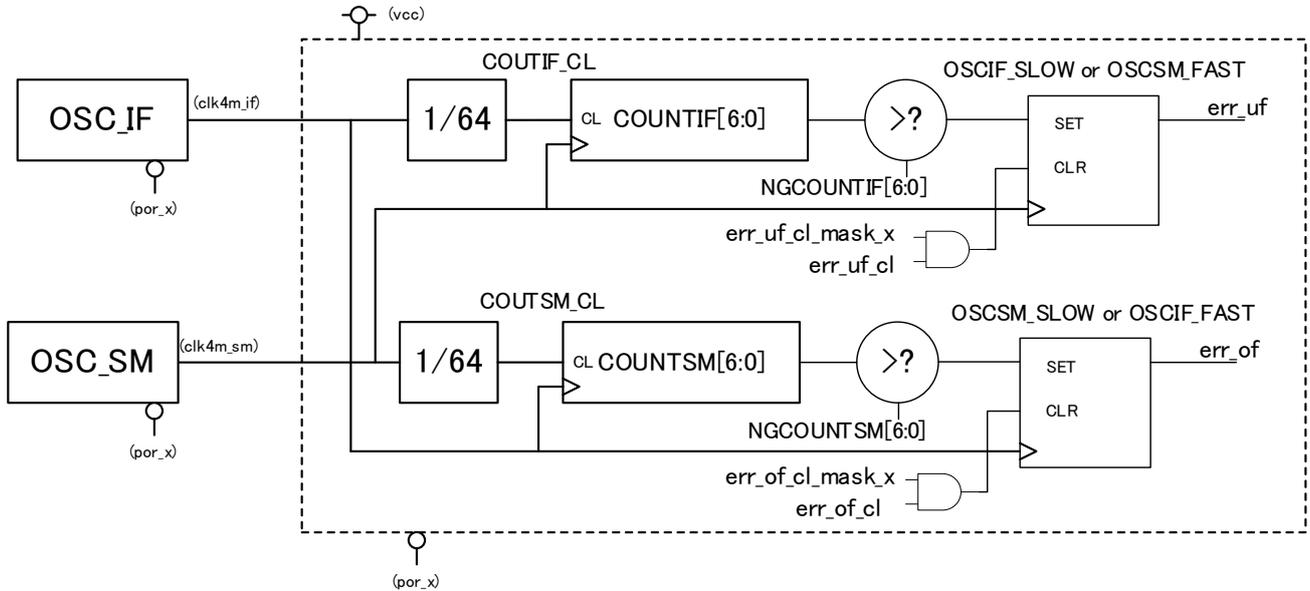
**Fig. 7.5.10-a Circuit diagram for two-way internal frequency monitoring**
