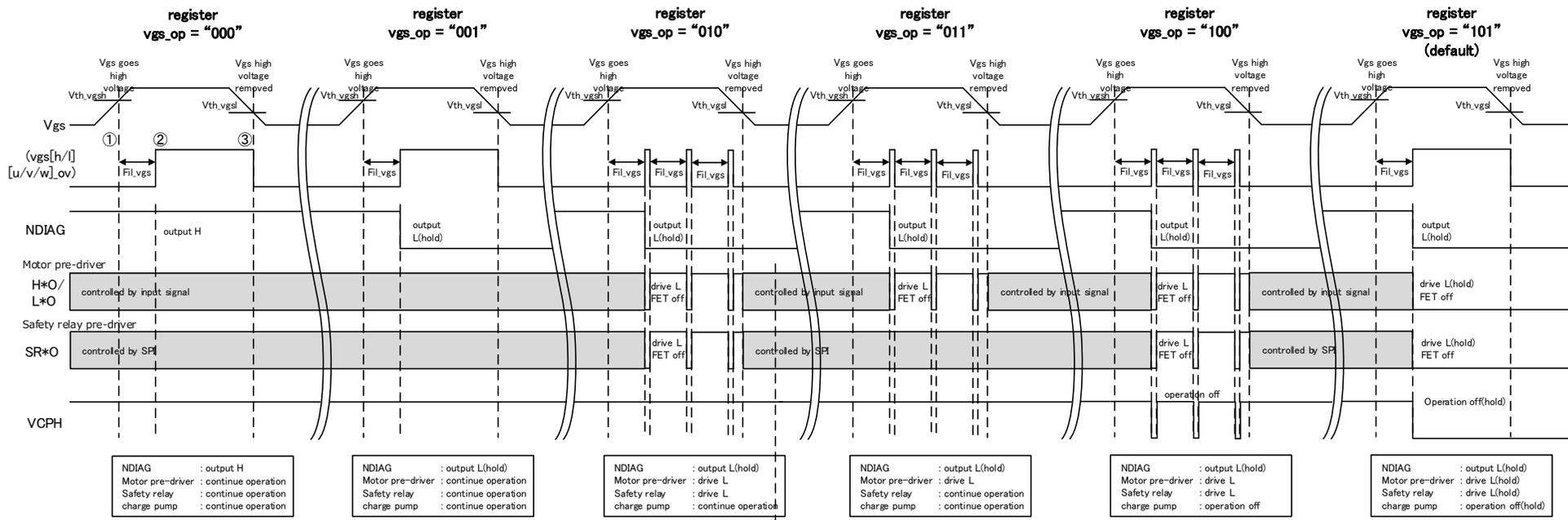
When register  $vgs[h/l][u/v/w]_{ov}$  is cleared via the SPI, NDIAG changes to "H."
