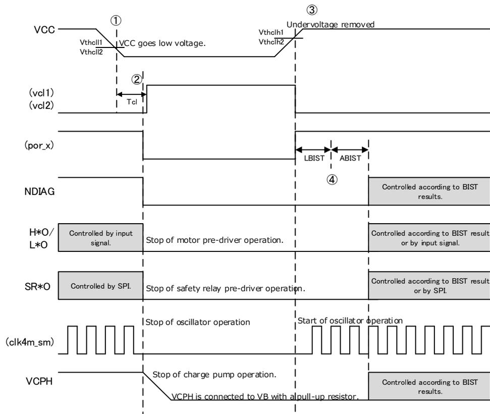
**Fig. 7.5.1-b Timing chart for VCC undervoltage detection**
