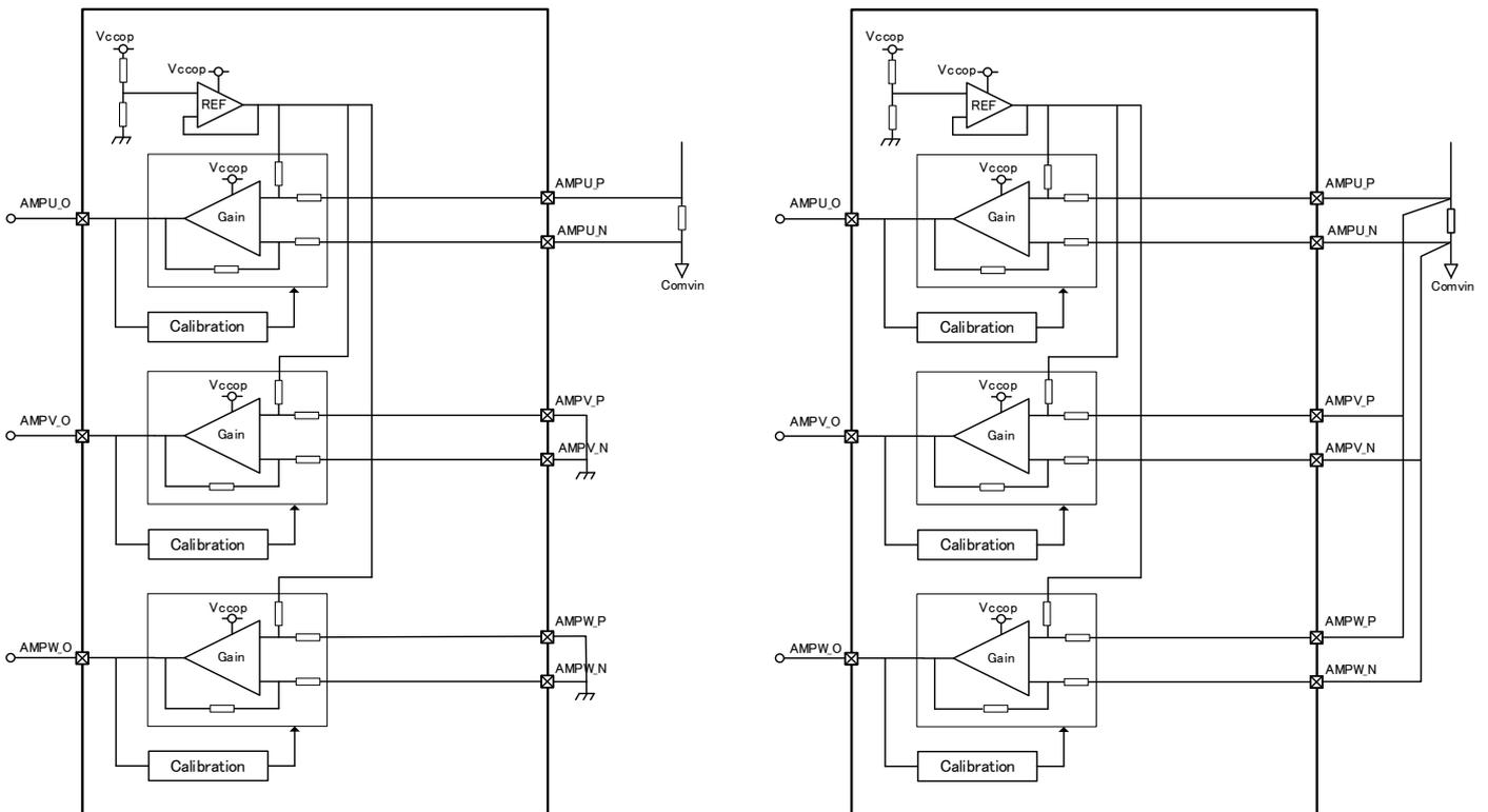
Fig. 7.3-b Block diagram for motor current detector circuit (single shunt)
