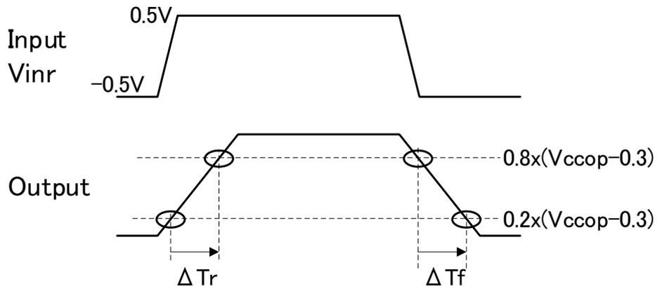
**Fig. 9-h Slew rate timing**
