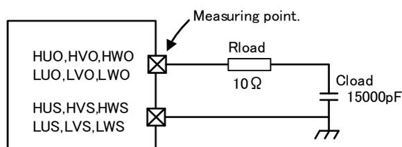
**Fig. 9-d Measurement circuit diagram (high side/low side)**
