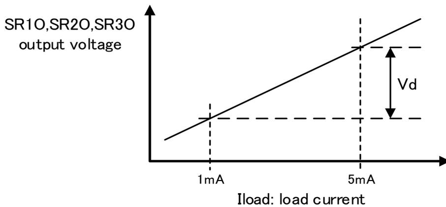
**Fig. 9-f** How to measure SR10,SR20,SR30 output resistance
