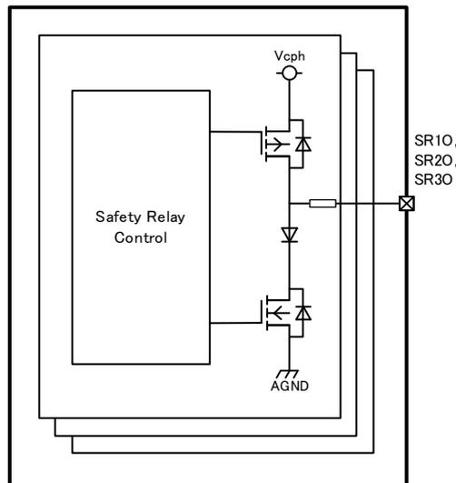
**Fig. 7.2-c Block diagram for safety relay circuit**
