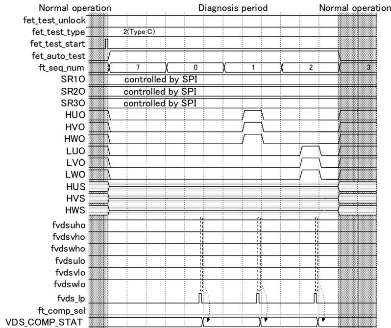
Fig. 7.8-e Operation waveforms in the inspection method Type C
