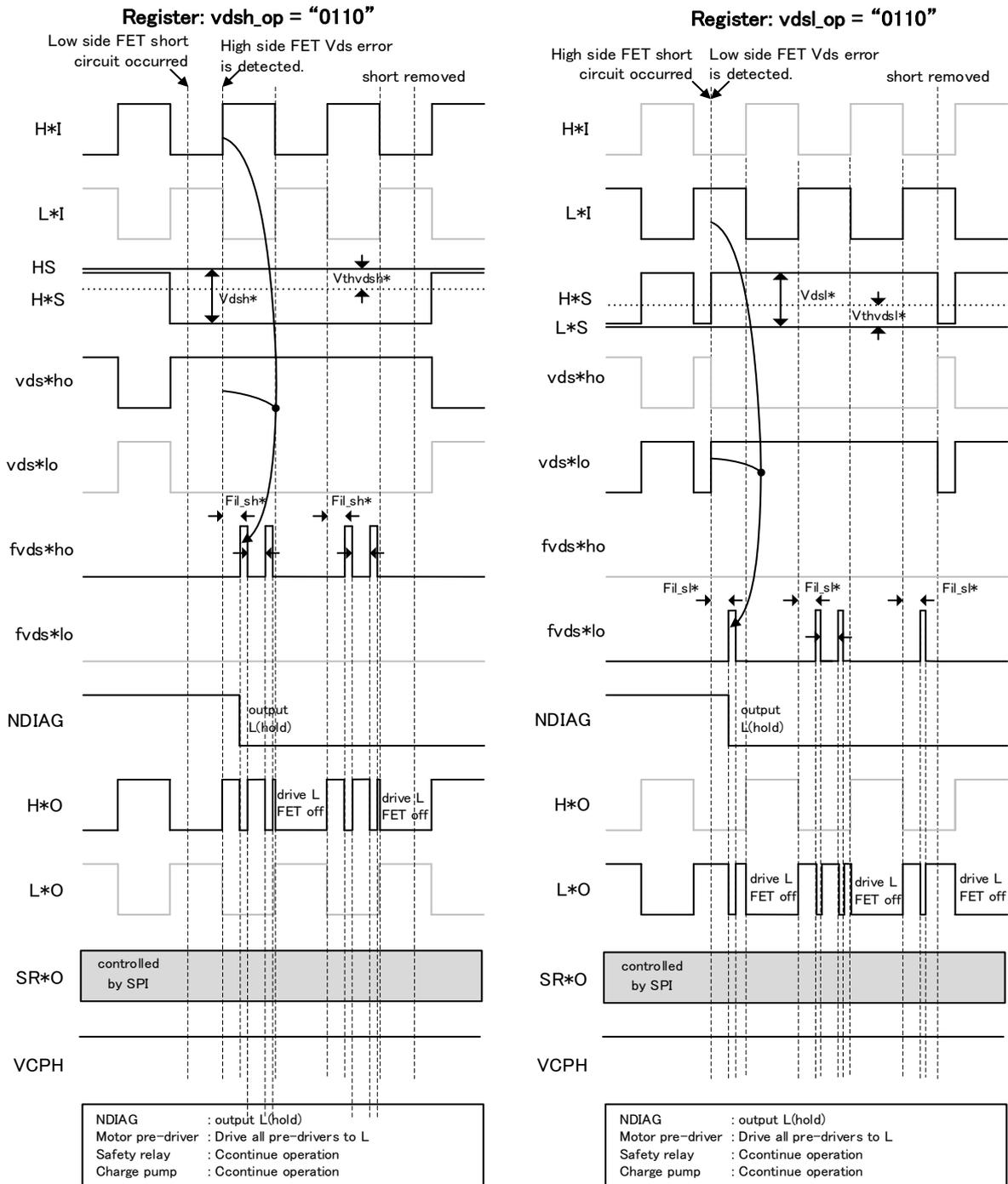
Fig. 7.5.8-h Timing chart for short-circuit detection (register vds\_l\_op = vds\_op "0110")
