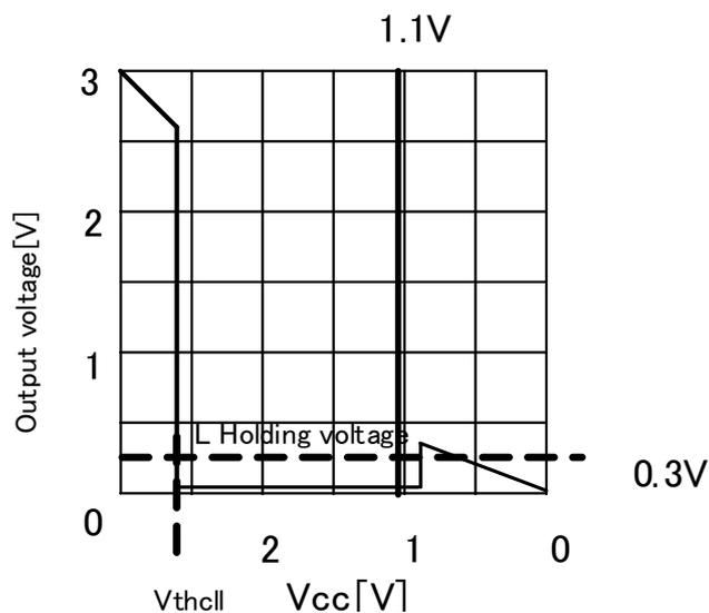
Fig. 9-i L Holding voltage
