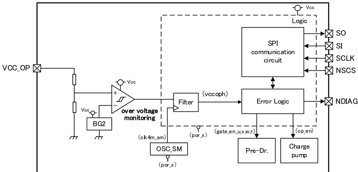
**Fig. 7.5.6-a Block diagram for VCC\_OP overvoltage detection**
