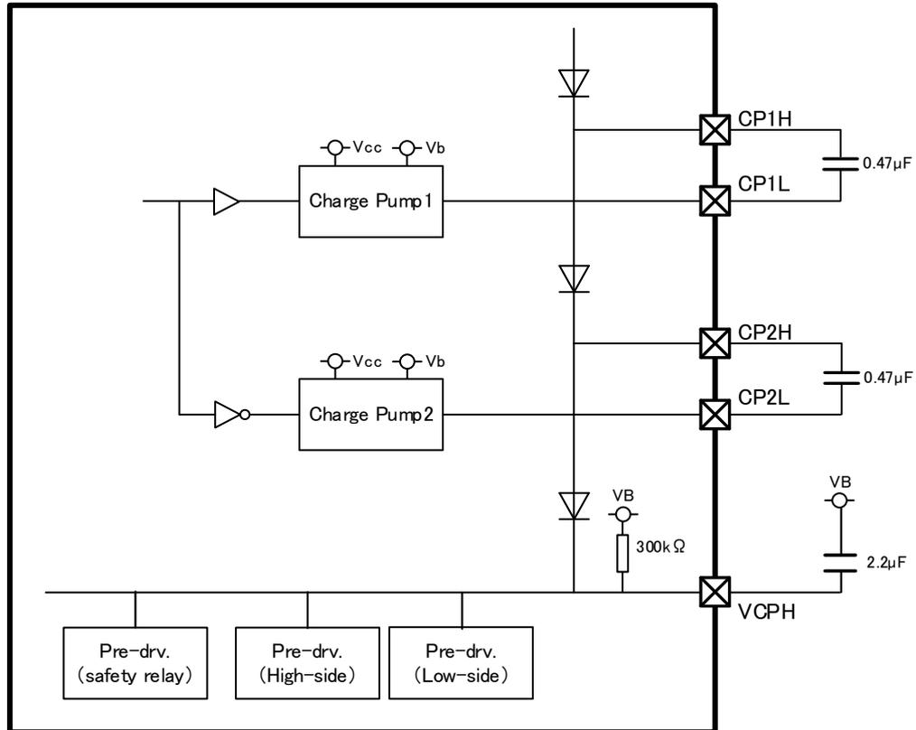
Fig. 9-a Charge pump application circuit diagram
