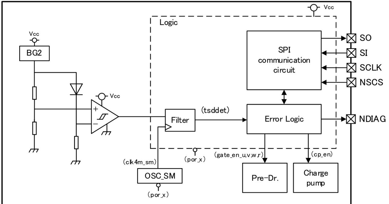
**Fig. 7.5.7-a Overtemperature detection block diagram**
