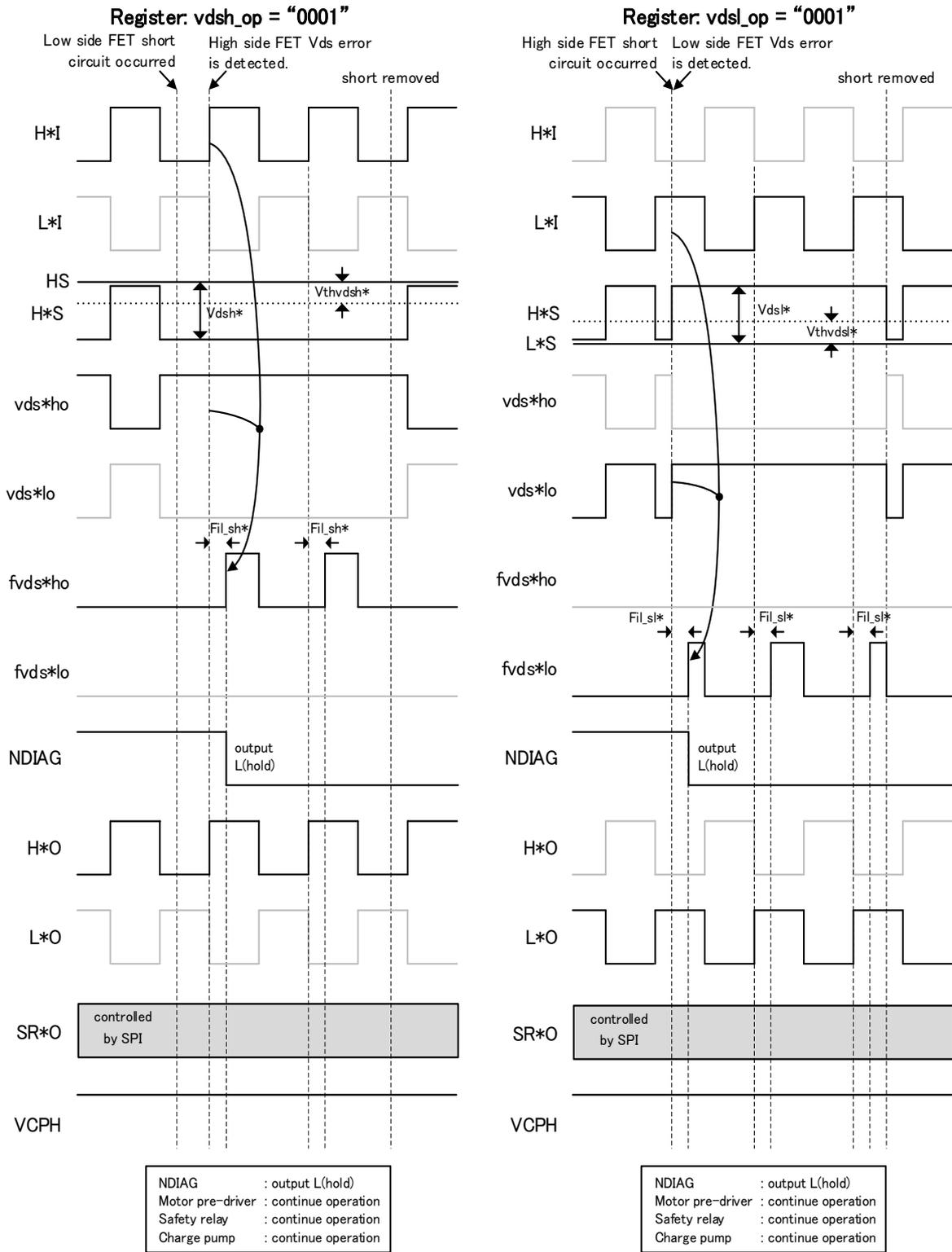
Fig. 7.5.8-c Timing chart for short-circuit detection (register vds\_op = vds\_op "0001")
