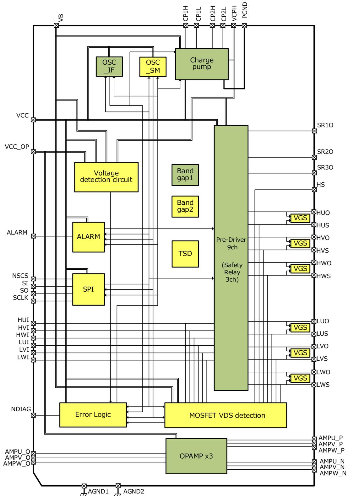
Note Functional blocks and wiring scheme have been simplified for the purpose of clarity (including individual block diagrams)
