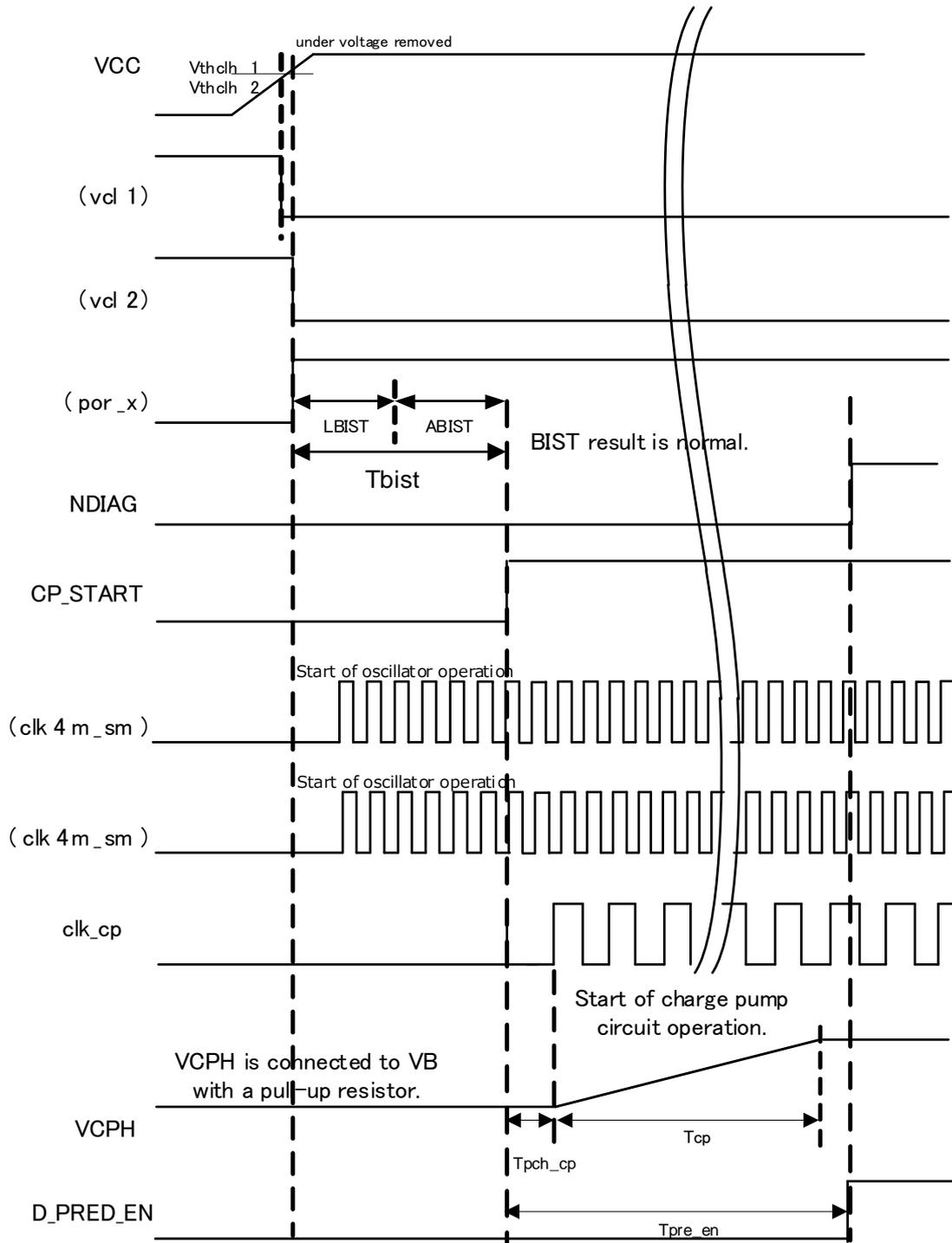
Fig. 9-b Charge pump circuit timing chart
