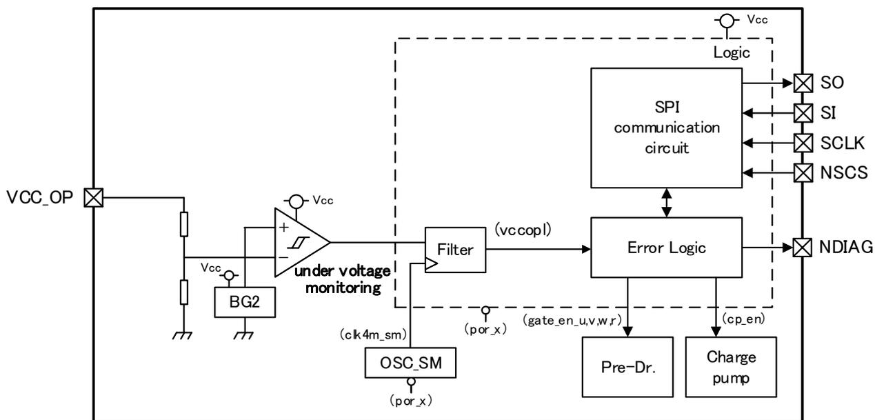
**Fig. 7.5.5-a Block diagram for VCC\_OP undervoltage detection**
