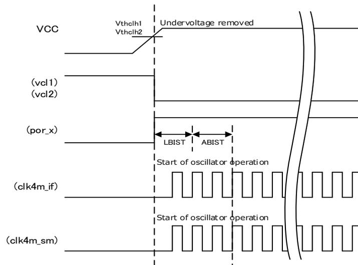
**Fig. 7.4-b Oscillator circuit timing chart**
