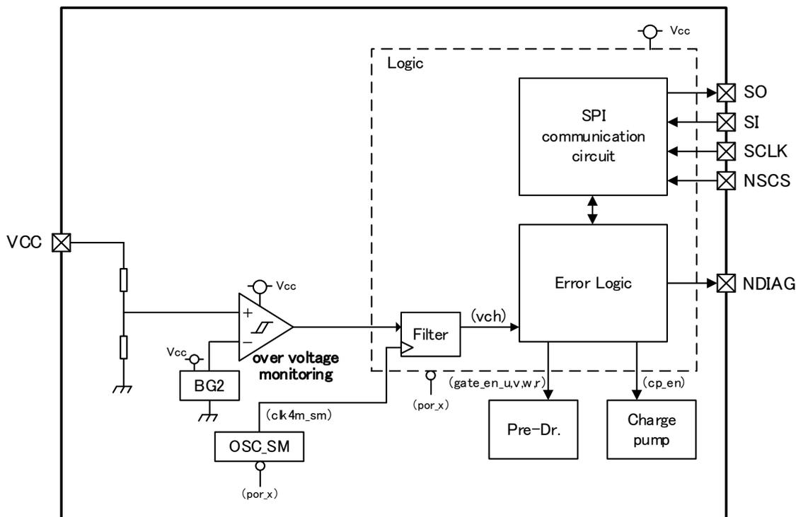
Fig. 7.5.4-a Block diagram for VCC overvoltage detection
