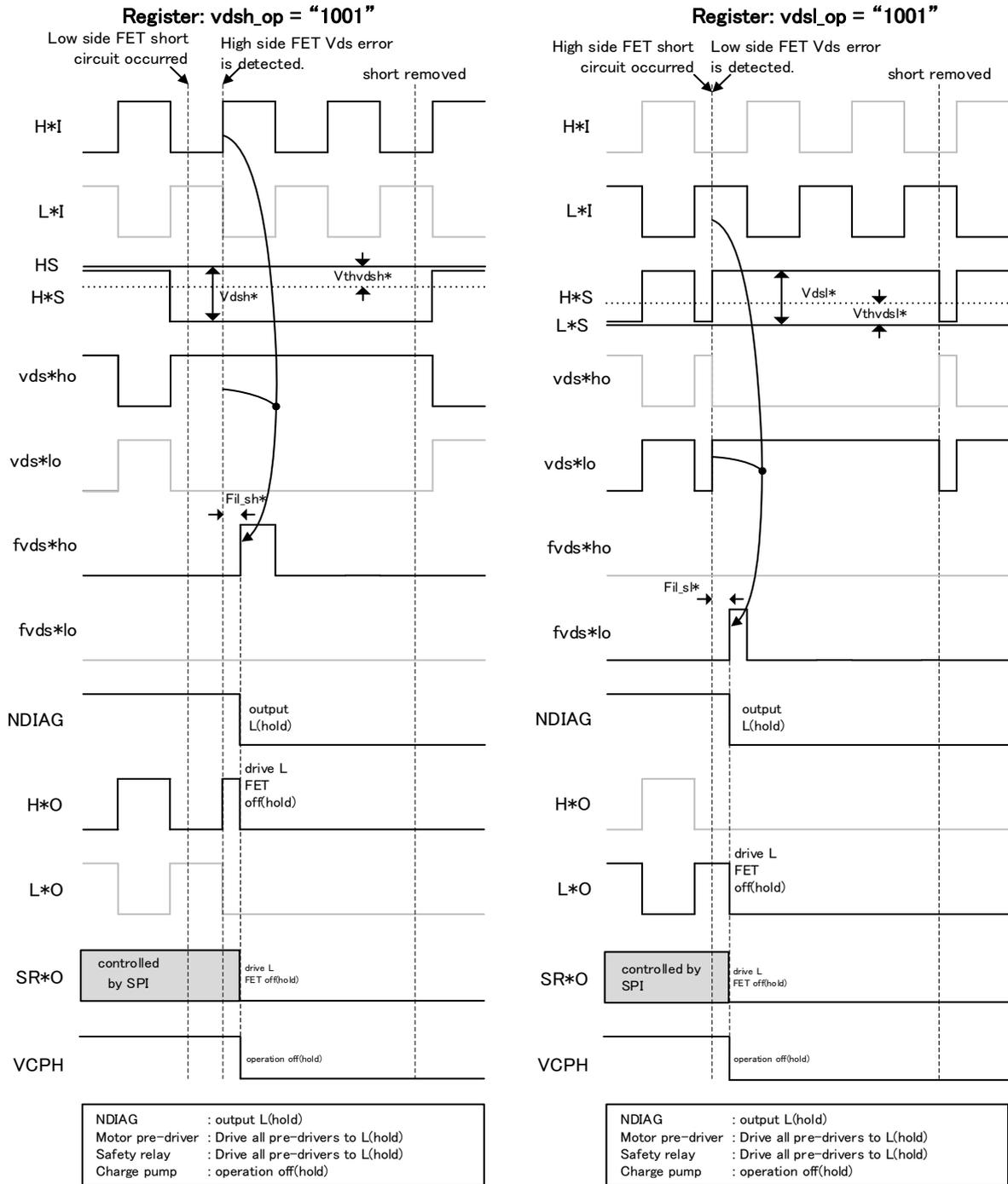
**Fig. 7.5.8-k Timing chart for short-circuit detection (register vds<sub>l</sub>\_op = vds<sub>h</sub>\_op "1001")**
