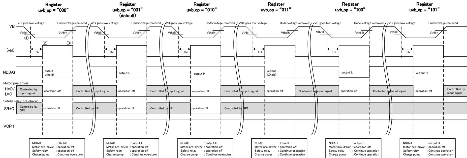
Fig. 7.5.2-b Timing chart for VB undervoltage detection
