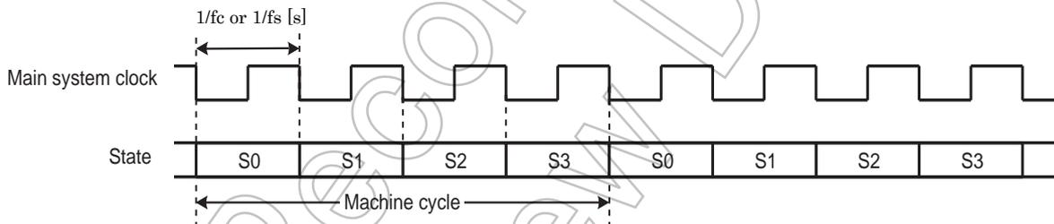
Figure 2-5 Machine Cycle
