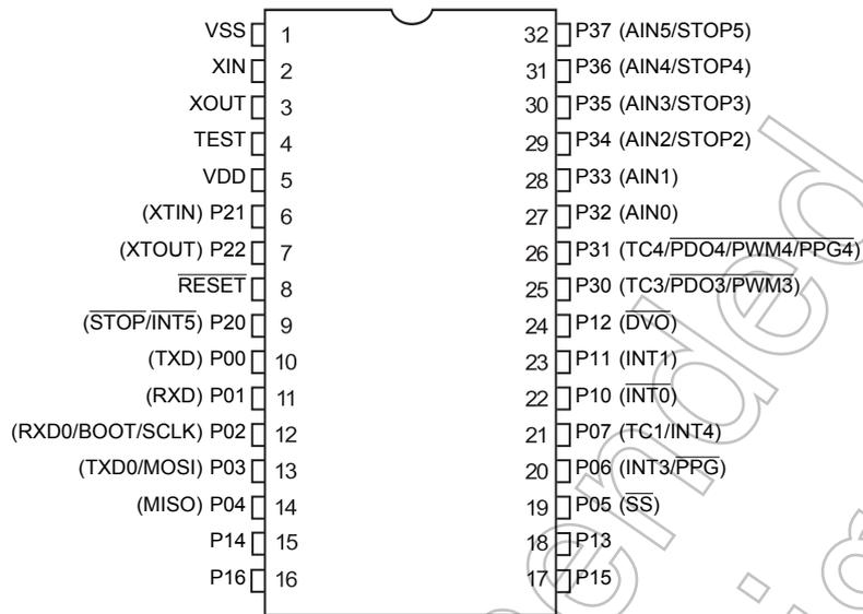
Figure 1-1 Pin Assignment
