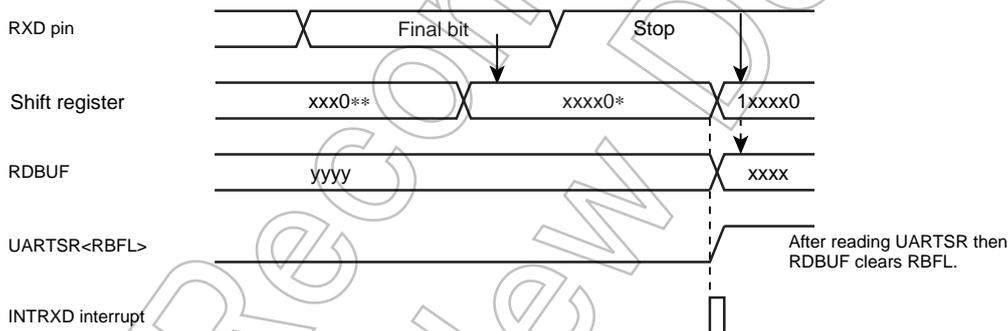
Figure 10-8 Generation of Receive Data Buffer Full
