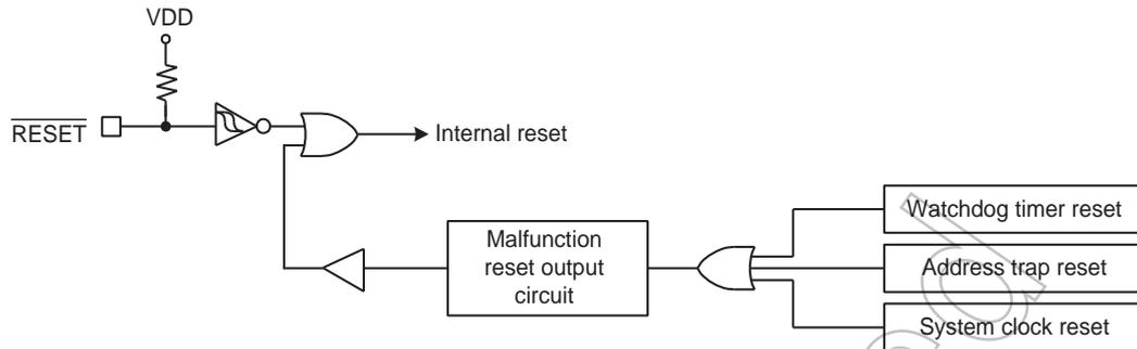
Figure 2-15 Reset Circuit
