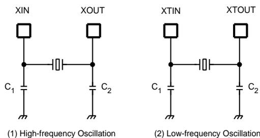
Note 1: To ensure stable oscillation, the resonator position, load capacitance, etc. must be appropriate. Because these factors are greatly affected by board patterns, please be sure to evaluate operation on the board on which the device will actually be mounted.
