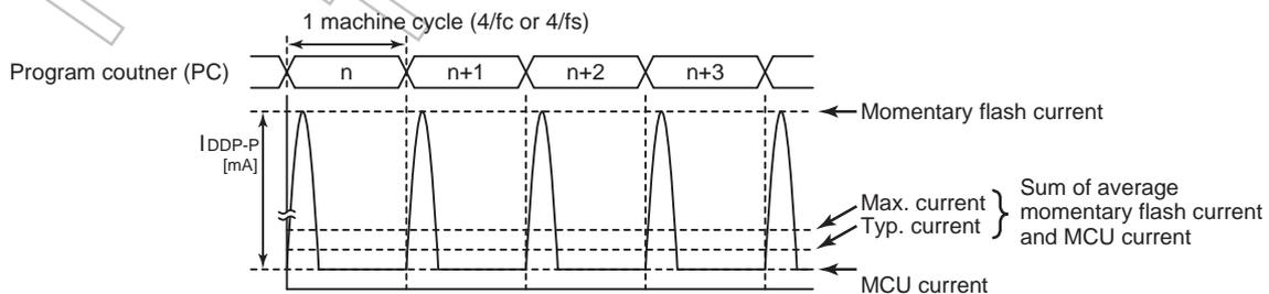
Figure 17-1 Intermittent Operation of Flash Memory
