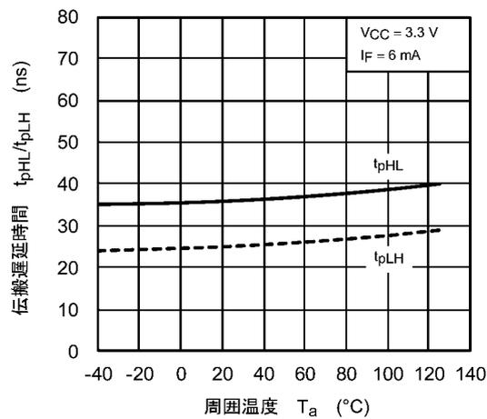
図 12.2.9  $t_{pHL}/t_{pLH} - T_a$
