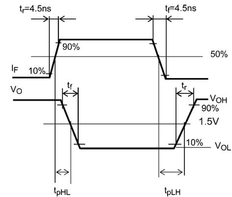
Fig. 12.1.5 Switching Time Test Circuit and Waveform
