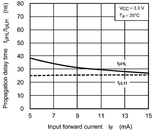
Fig. 12.2.13  $t_{pHL}/t_{pLH} - I_F$
