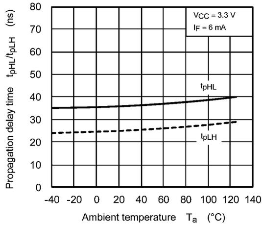
Fig. 12.2.9  $t_{pHL}/t_{pLH} - T_a$
