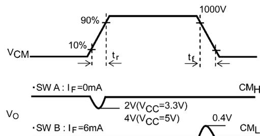
$$C_{M_L} = \frac{800(\text{V})}{t_r(\mu\text{s})} \quad C_{M_H} = -\frac{800(\text{V})}{t_f(\mu\text{s})}$$
