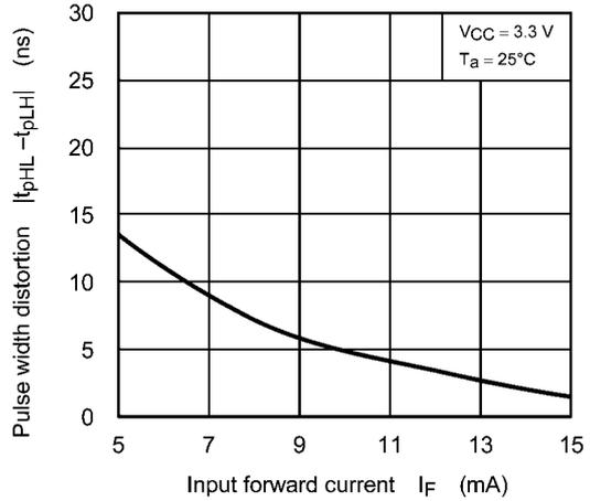
Fig. 12.2.14  $|t_{pHL} - t_{pLH}| - I_F$
