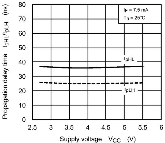
Fig. 12.2.17  $t_{pHL}/t_{pLH} - V_{CC}$
