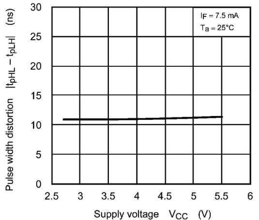
Fig. 12.2.18  $|t_{pHL} - t_{pLH}| - V_{CC}$
