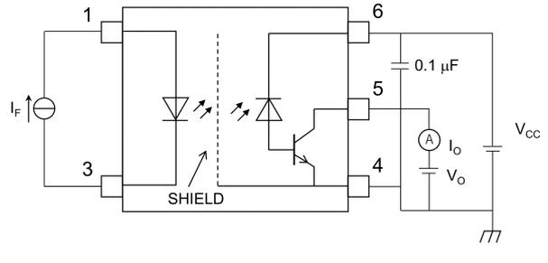
Fig. 12.1.4  $I_O$  Test Circuit
