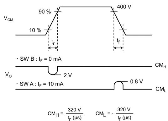
Fig. 12.1.6 Common-Mode Transient Immunity Test Circuit and Waveform
