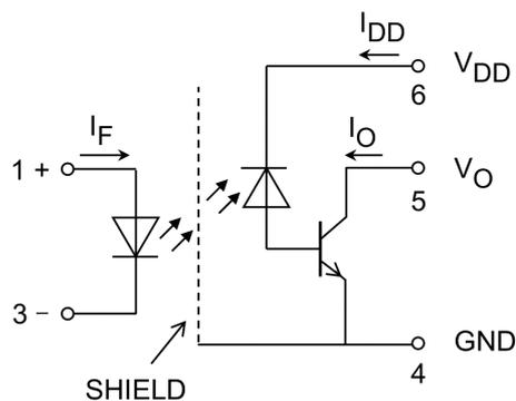
Note: A 0.1- $\mu$ F bypass capacitor must be connected between pin 6 and pin 4.
