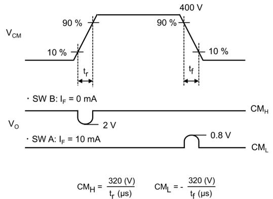
Fig. 12.1.6 Common-Mode Transient Immunity Test Circuit and Waveform
