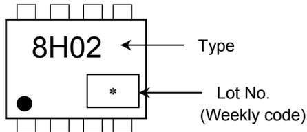
Note 4: The mark "●" on the lower left of the marking indicates Pin 1.
