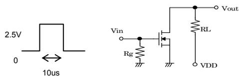
Gate Pulse Width  $10\ \mu\text{ s}$ ,  $t_r, t_f < 5\text{ ns}$
