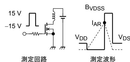
$$E_{AS} = \frac{1}{2} \cdot L \cdot I^2 \cdot \left( \frac{B_{VDSS}}{B_{VDSS} - V_{DD}} \right)$$
