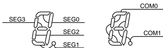
Figure 16-7 Example of COM, SEG Pin Connection
