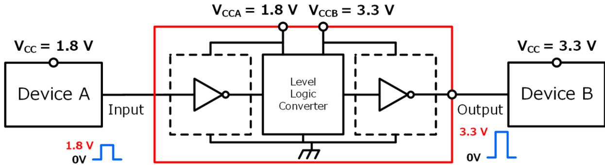
**Figure 10 Example of up translation using a dual-supply dedicated level shifter IC (TC7SP3125)**
