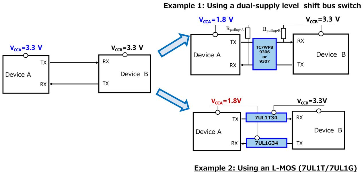
**Figure 17 Example of level-shifting for a two-line UART interface**
