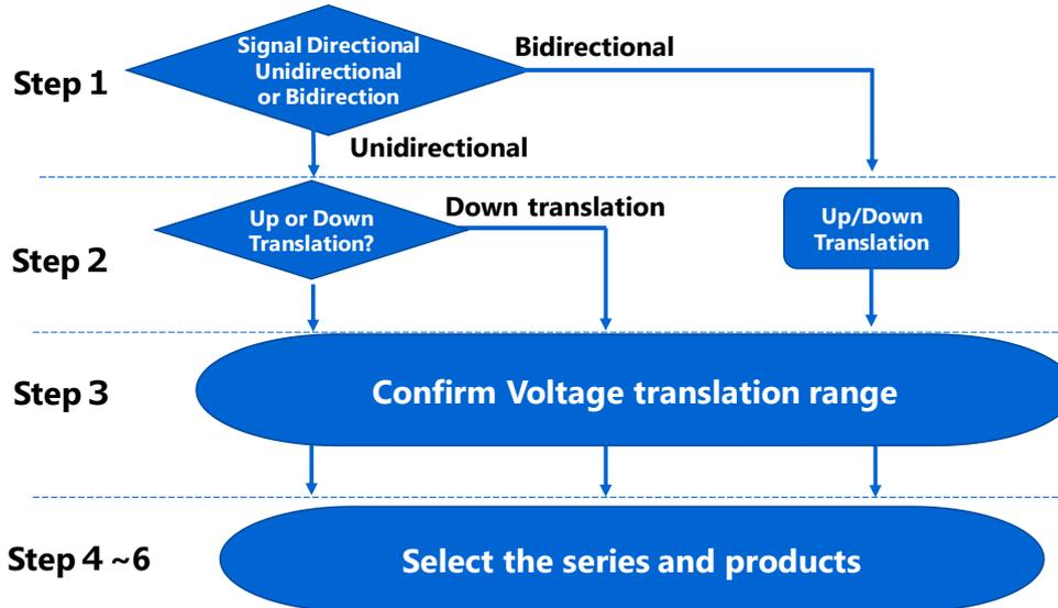
**Figure 6 Steps for selecting a level shifter**
