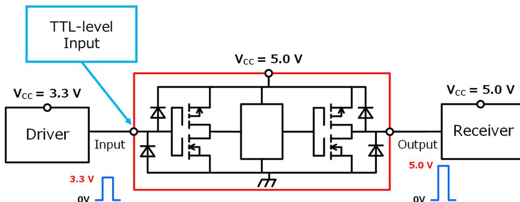
**Figure 7 Example of up translation using an IC with a TTL-level input**
