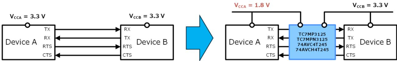
**Figure 16 Example of level-shifting for a four-line UART interface**
