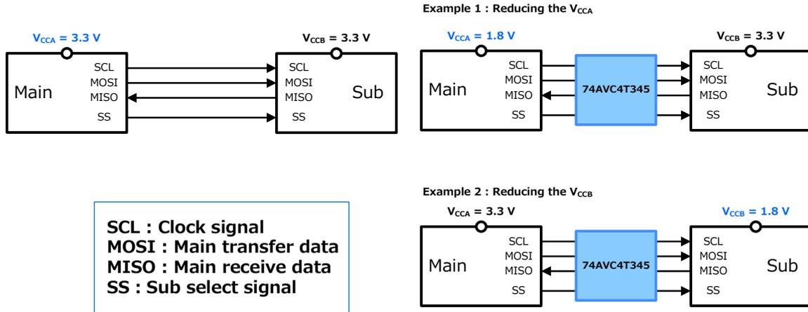
**Figure 19 Examples of level-shifting for an SPI interface**
