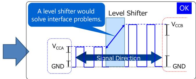
**Figure 1 Why are level shifters necessary?**
