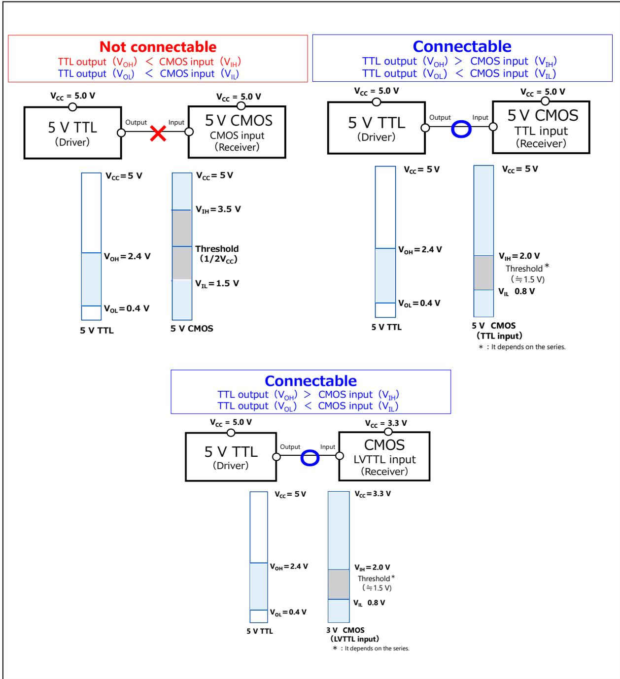
**Figure 2 TTL-level inputs (5-V TTL and 3.3-V LVTTTL)**
