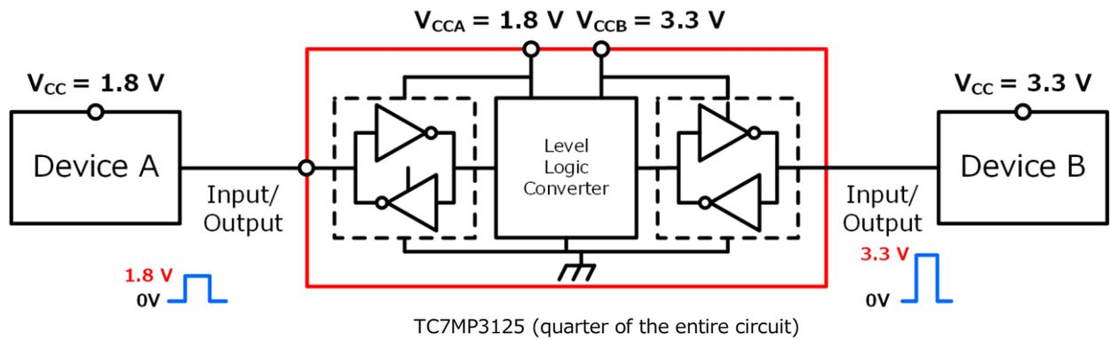
**Figure 13 Case 7: Example of up/down translation using a dual-supply bidirectional dedicated level shifter IC (buffer-type) (TC7MP3125)**
