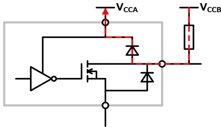
**Figure 4 IC without an output-tolerant function (power-down protection)**
