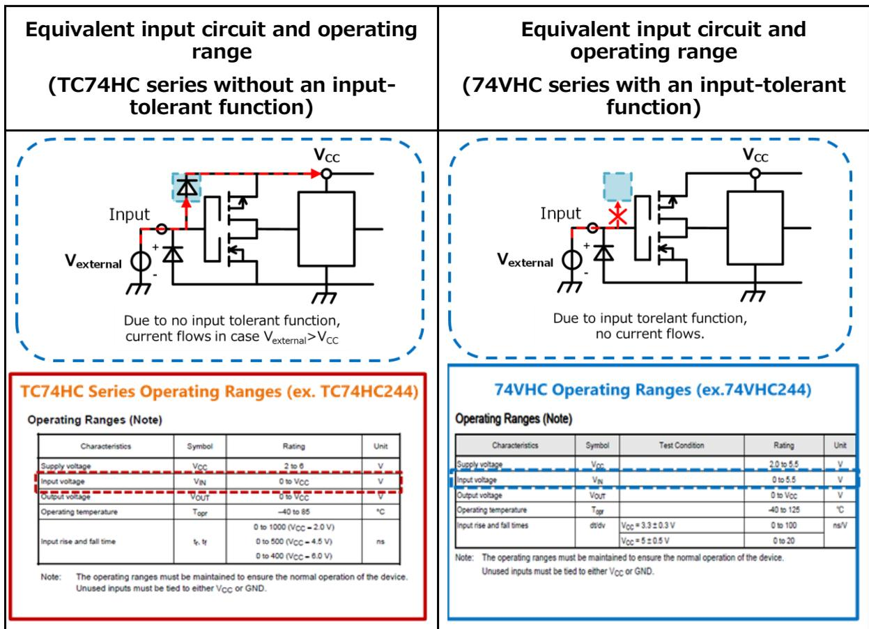
Figure 3 Equivalent input circuits and operating ranges of ICs with and without an input-tolerant function
