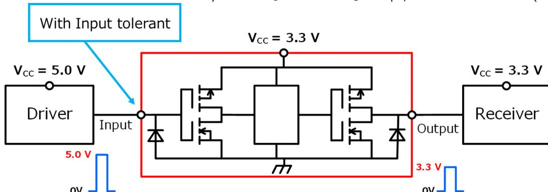
**Figure 11 Example of down translation using an IC with an input-tolerant function(TC7SZ34)**
