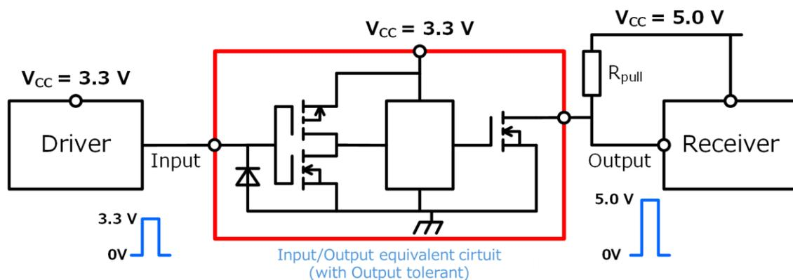
**Figure 8 Example of up translation using an IC with an open-drain output (74LCX05)**
