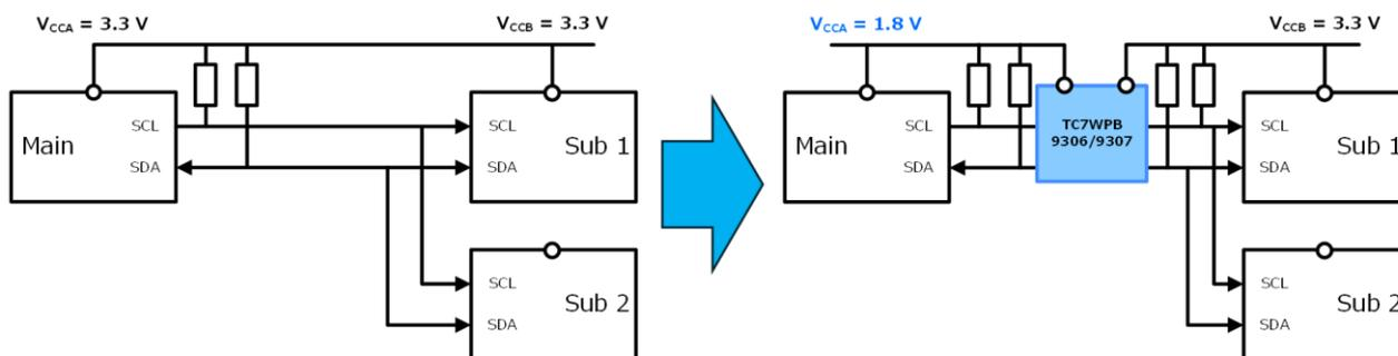
**Figure 18** Example of level-shifting for an I<sup>2</sup>C interface
