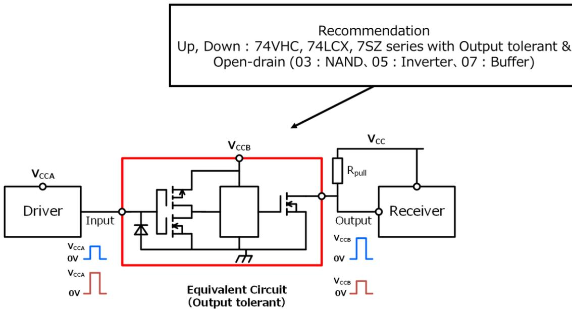
Figure 5 Examples of up and down translation using ICs with an open-drain output
