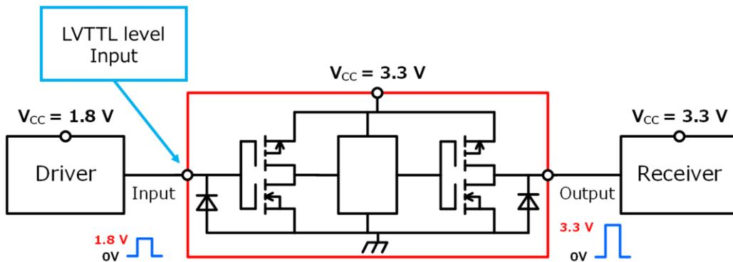
**Figure 9 Example of up translation from ultralow voltage using an IC with an LVTTTL-level input (7UL1T34)**
