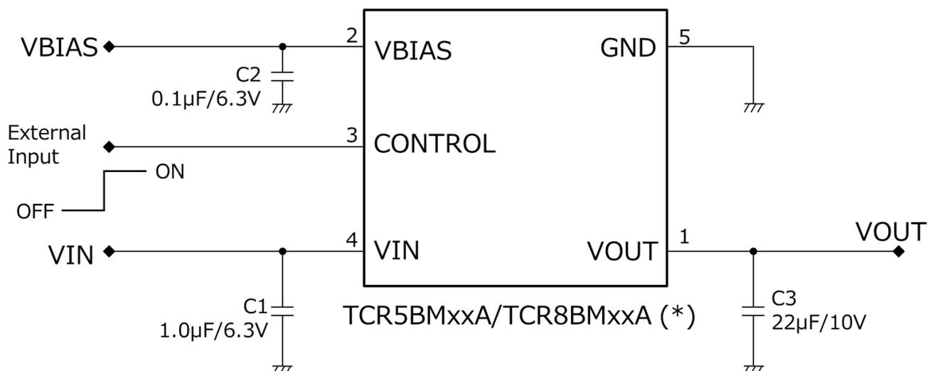
Figure 3.1 Applied Circuits for TCR5BM/TCR8BM Series RF Blocks
