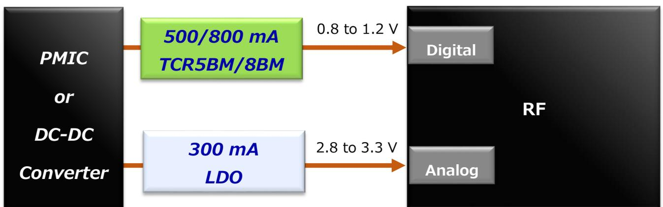
Figure 2.1 RF Block Power Configuration
