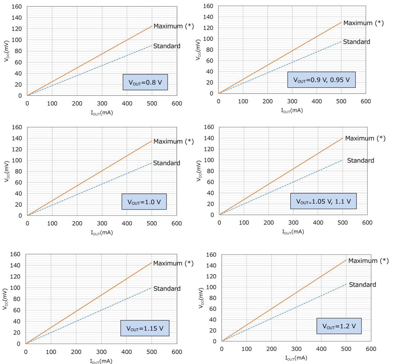
**Figure 4.2 Dropout Voltage Characteristics of TCR5BM Series ( $V_{BIAS}=3.3$  V,  $V_{OUT}=0.8$  to  $1.2$  V)**
