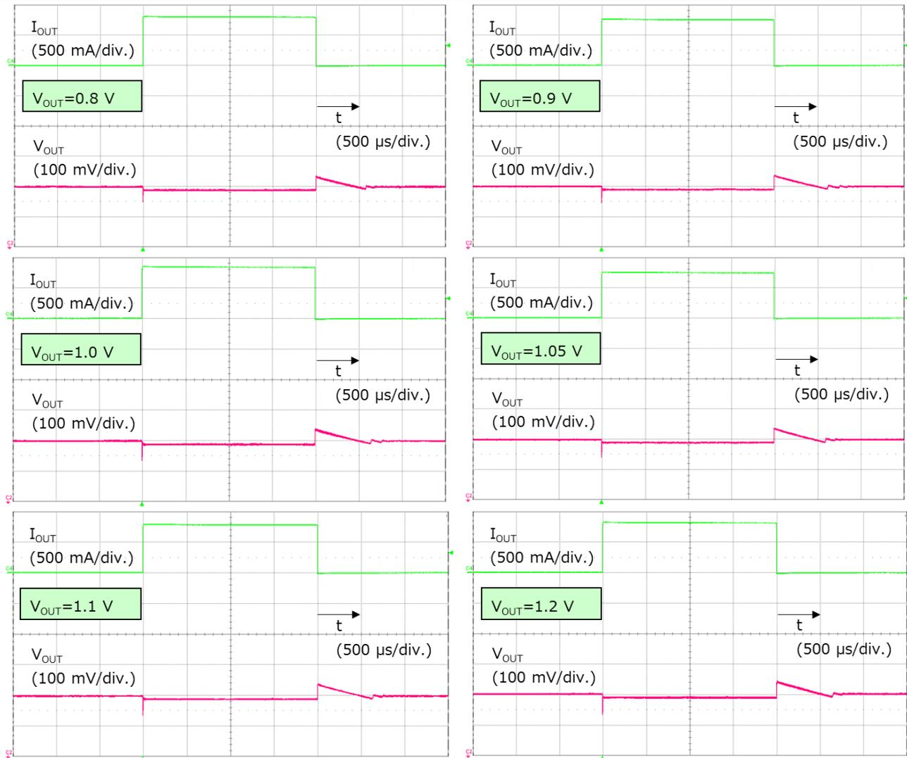
**Figure 4.5 Load Transient Responses of TCR8BM Series**
