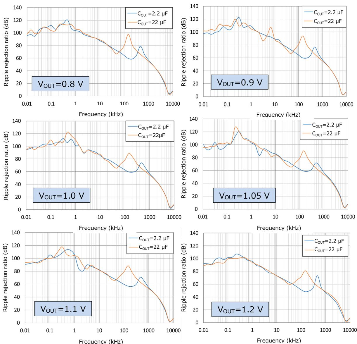
**Figure 4.6 Ripple Rejection Ratio Frequency Characteristics of TCR5BM Series**
