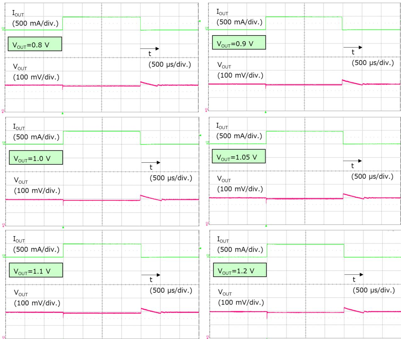
**Figure 4.4 Load Transient Responses of TCR5BM Series**
