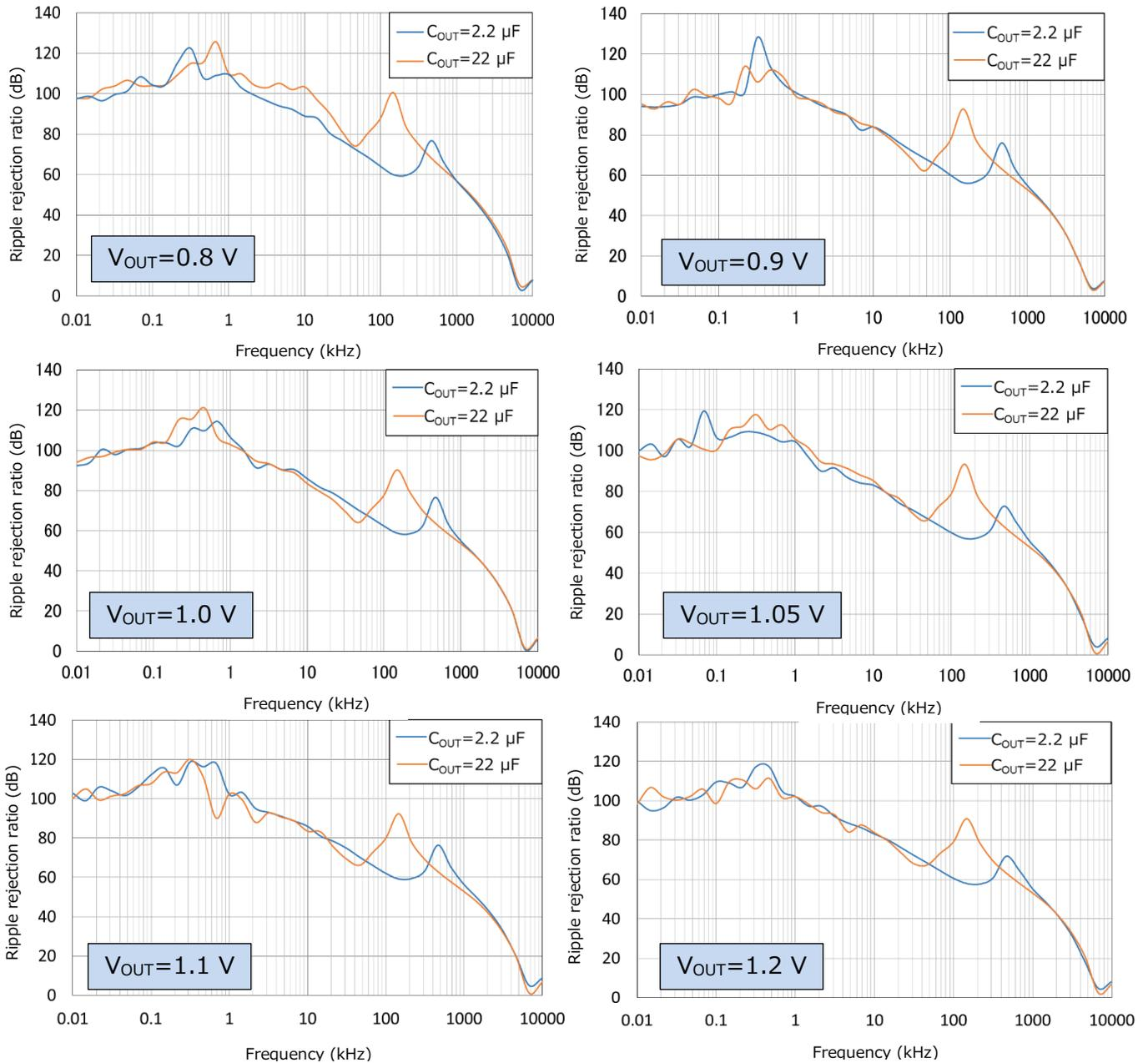
**Figure 4.7 Ripple Rejection Ratio Frequency Characteristics of TCR8BM Series**
