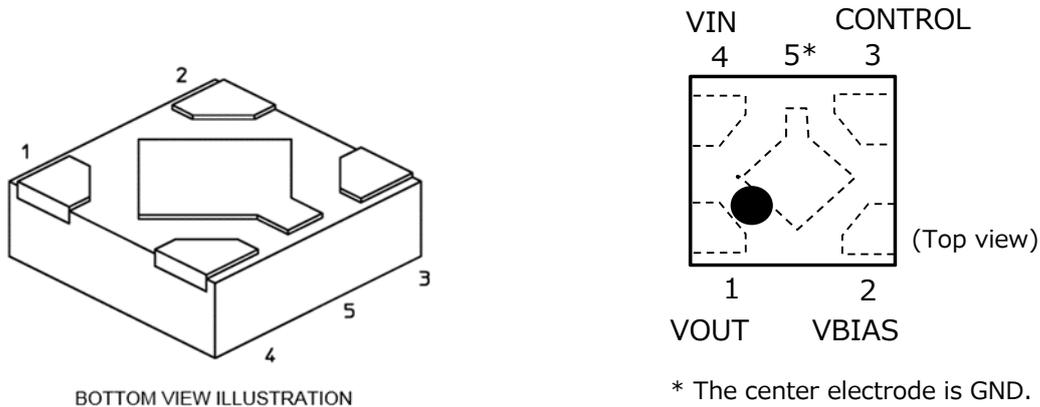
Figure 5.1 Appearance and Pin Layout of TCR5BM/8BM Series
