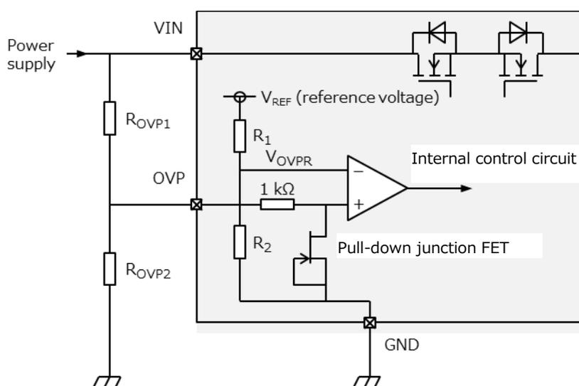
**Figure 6.1 OVP circuit**
