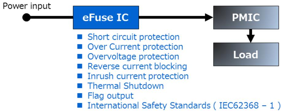
**Figure 2.1 Application example of an eFuse IC**
