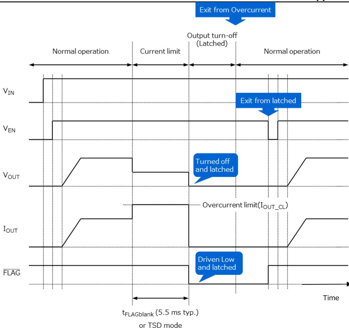
**Figure 6.7 Example of an OCP operation**
