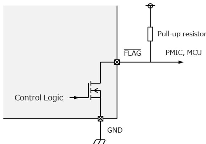
**Figure 6.17 Equivalent circuit of the  $\overline{\text{FLAG}}$  pin**
