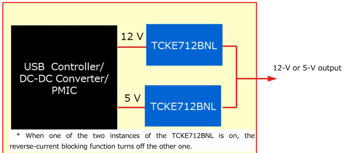
**Figure 8.5 Using two instances of the TCKE712BNL as a power multiplexer for a USB device**
