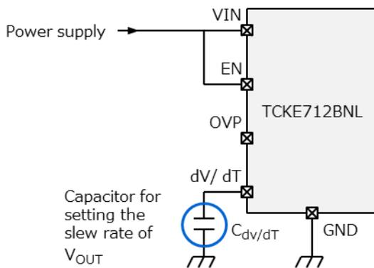
**Figure 6.14 Capacitor connected to the dV/dT input**
