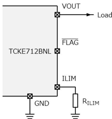
**Figure 6.9 Resistor connected to the ILIM input**
