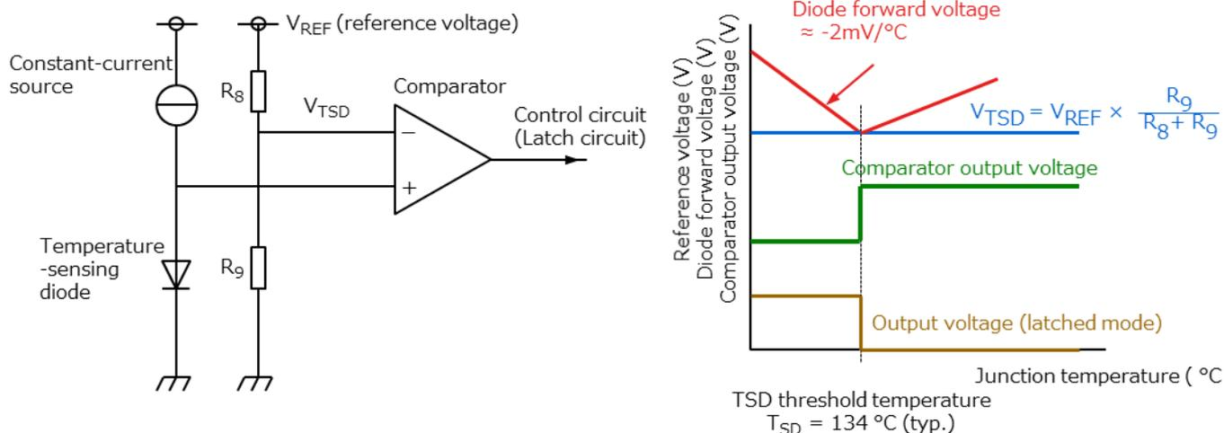
**Figure 6.6 TSD circuit and its principle of operation**
