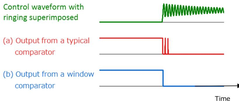
**Figure 6.19** Outputs from a typical comparator and a window comparator
