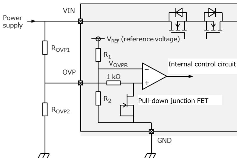
**Figure 6.1 OVP circuit**
