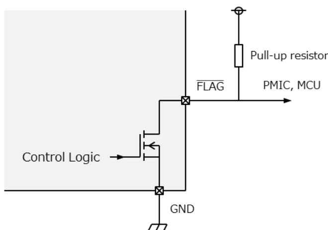
**Figure 6.17 Equivalent circuit of the  $\overline{FLAG}$  pin**
