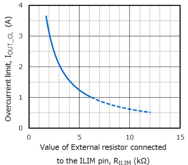
**Figure 6.10 Example of the  $I_{OUT\_CL}$  –  $R_{ILIM}$  curve**
