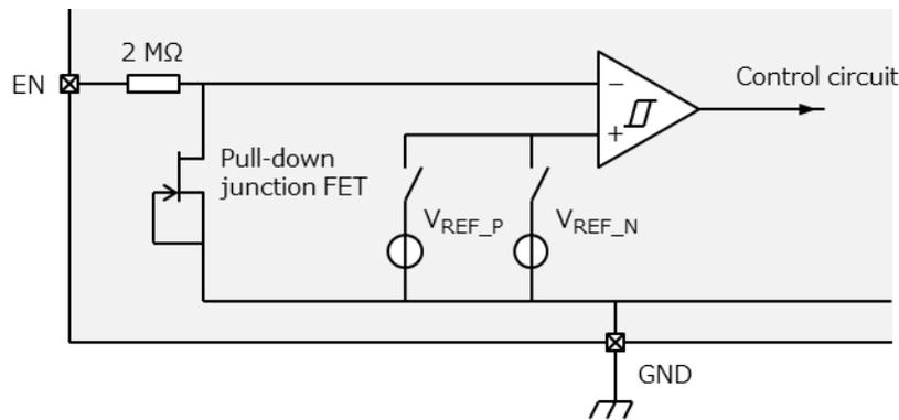
**Figure 6.18** Equivalent circuit of the EN pin
