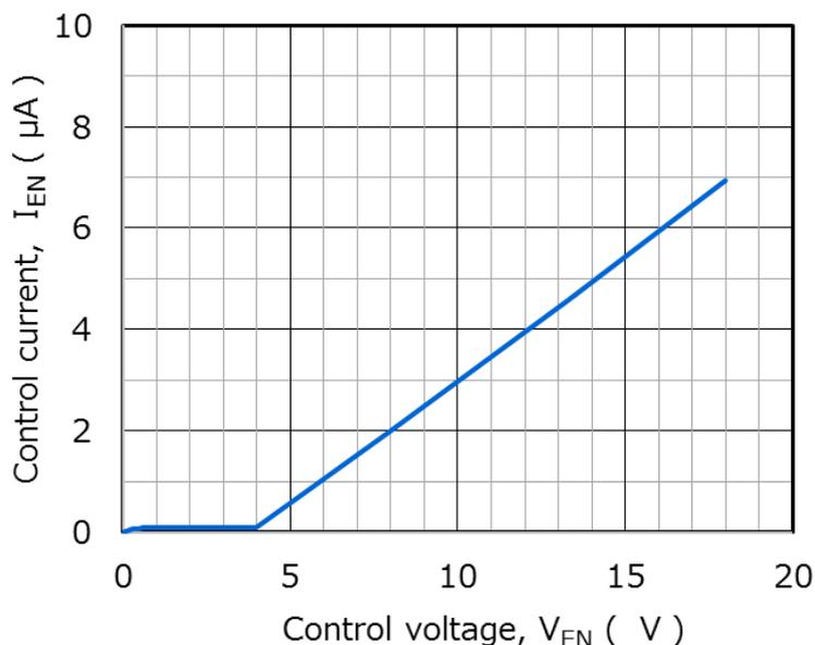
**Figure 6.20**  $I_{EN}$  -  $V_{EN}$  characteristics (shown only as a guide)
