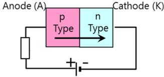
Schematic diagram of a diode
