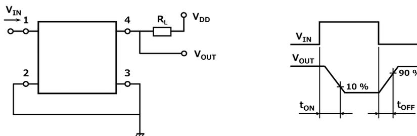
Fig. 11.1 Switching Time Test Circuit and Waveform
