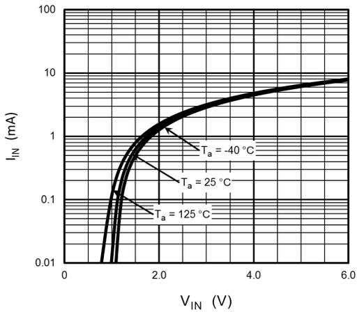
Fig. 12.1  $I_{IN} - V_{IN}$
