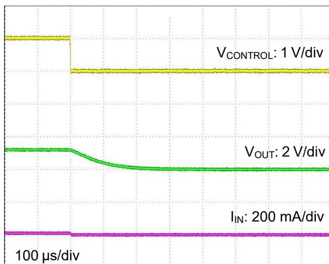
$V_{OUT} = 2.8 \text{ V}$
