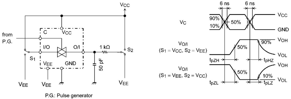
図1.  $t_{pLZ}$ ,  $t_{pHZ}$ ,  $t_{pZL}$ ,  $t_{pZH}$
