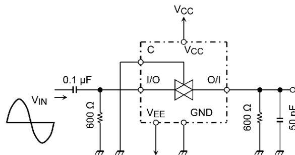
図4. Feedthrough Attenuation
