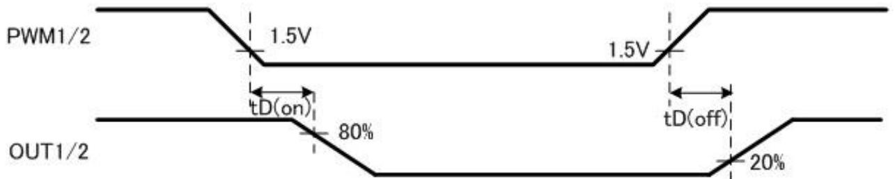
Figure 10.2. Driver output delay time
