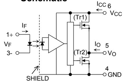
Note: A 0.1  $\mu$ F bypass capacitor must be connected between pins 6 and 4.
