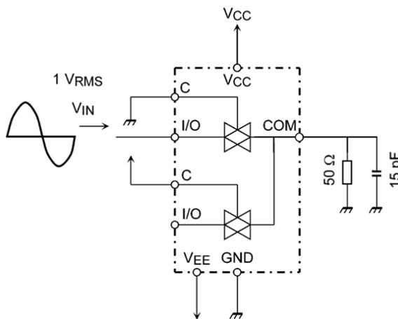
**Figure 6 Cross Talk (between any two switches)**
