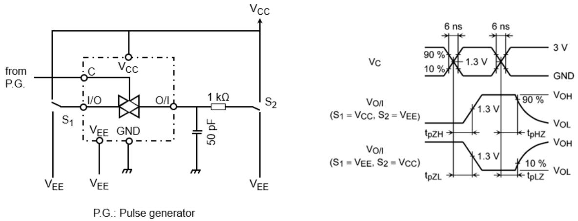
Figure 1  $t_{pLZ}$ ,  $t_{pHZ}$ ,  $t_{pZL}$ ,  $t_{pZH}$
