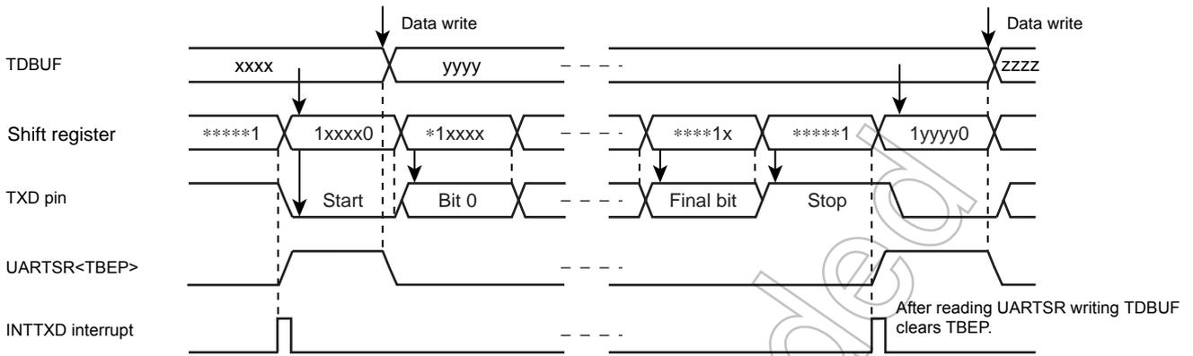
Figure 11-9 Generation of Transmit Data Buffer Empty
