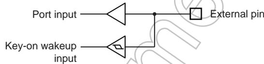
Figure 13-2 Key-on Wakeup Input and Port Input
