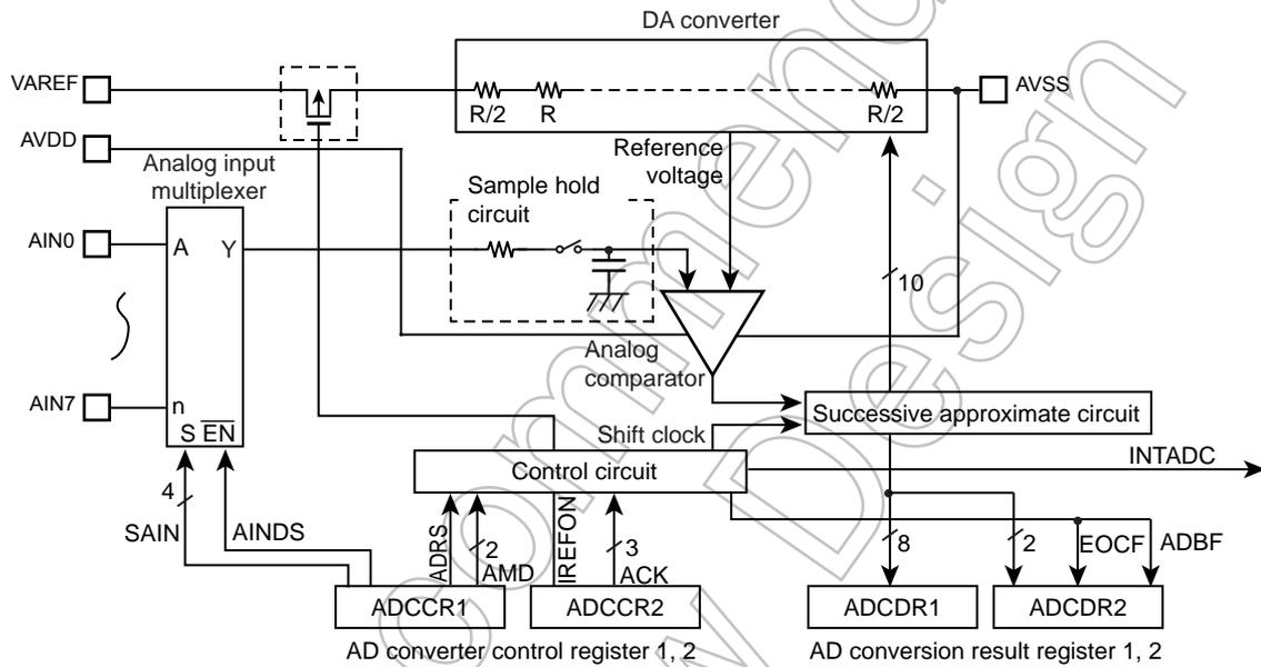
Note: Before using AD converter, set appropriate value to I/O port register combining a analog input port. For details, see the section on "I/O ports".
