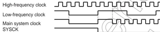
Example :Switching from the SLOW1 mode to the NORMAL2 mode (fc = 16 MHz, warm-up time is 4.0 ms).
