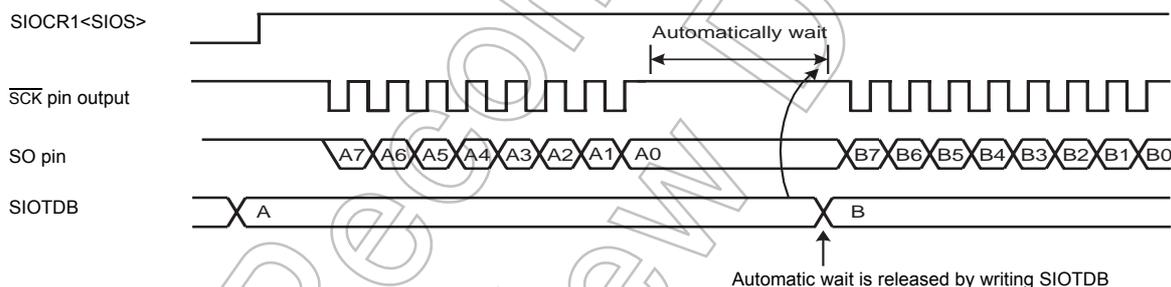
Figure 10-2 Automatic-wait Function (Example of transmit mode)
