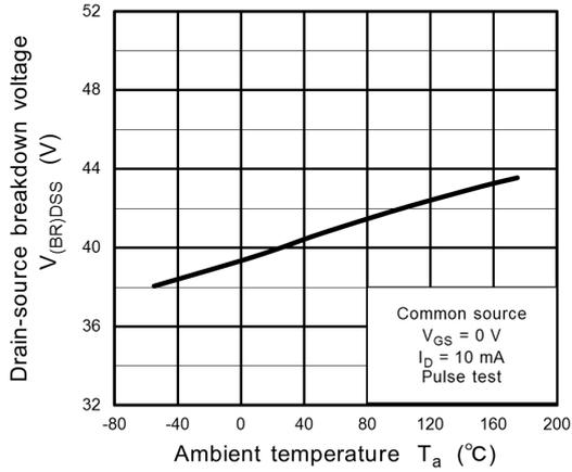
**Fig. 8.7**  $V_{(BR)DSS} - T_a$
