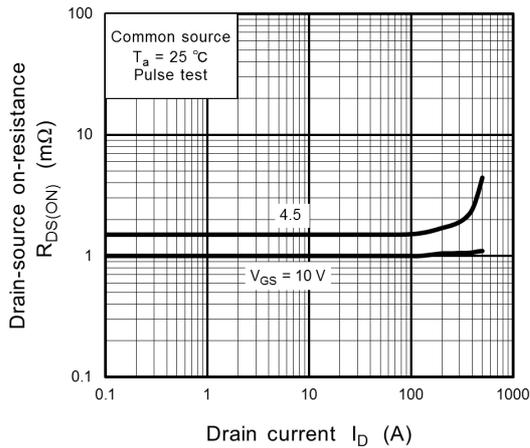
**Fig. 8.5  $R_{DS(ON)} - I_D$**
