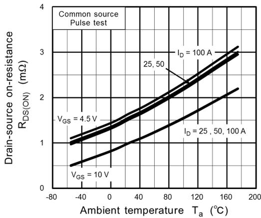
**Fig. 8.9**  $R_{DS(ON)} - T_a$
