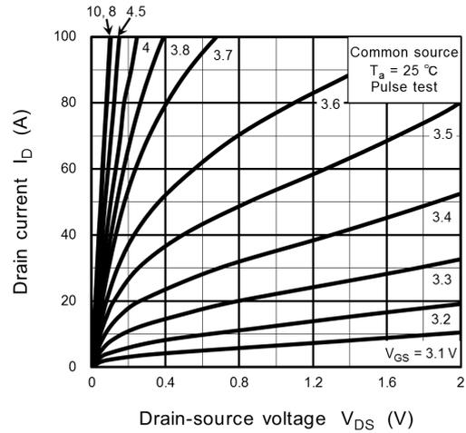
**Fig. 8.2  $I_D - V_{DS}$**
