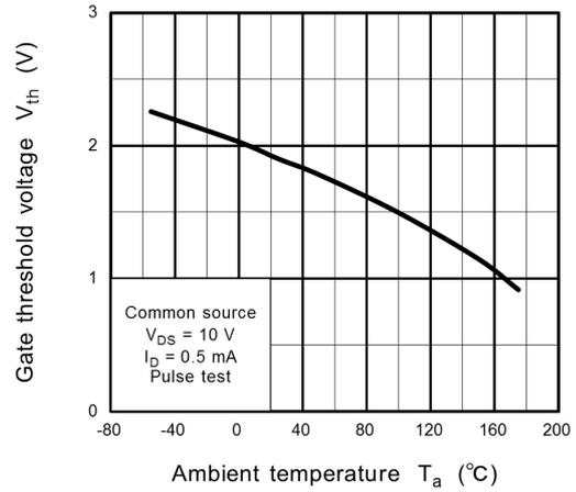
**Fig. 8.8**  $V_{th} - T_a$
