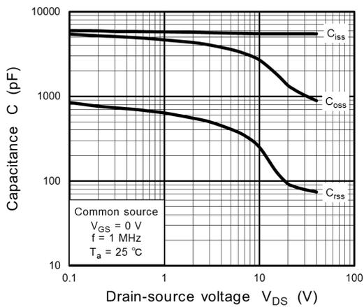
**Fig. 8.11** Capacitance -  $V_{DS}$
