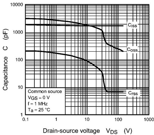
Fig. 8.11 Capacitance -  $V_{DS}$
