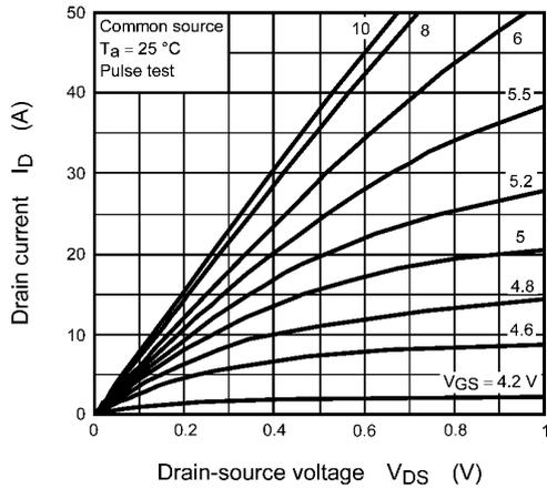
Fig. 8.1  $I_D - V_{DS}$
