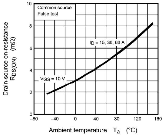
**Fig. 8.9**  $R_{DS(ON)} - T_a$
