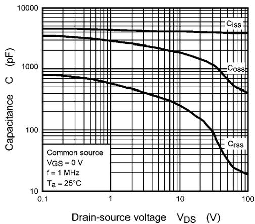
**Fig. 8.11** Capacitance -  $V_{DS}$
