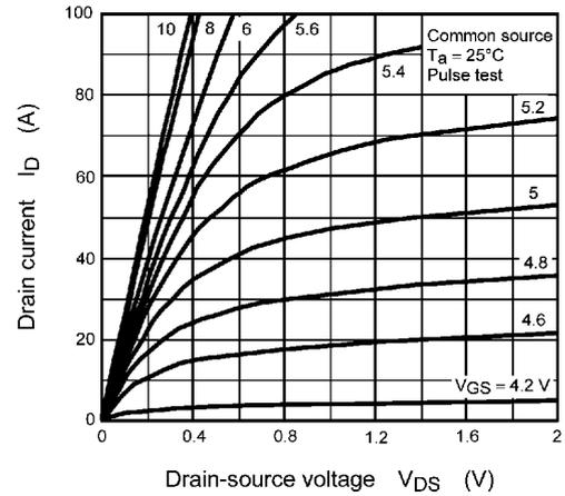
Fig. 8.2  $I_D - V_{DS}$
