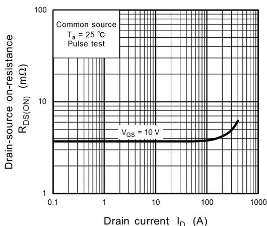
Fig. 8.5  $R_{DS(ON)} - I_D$
