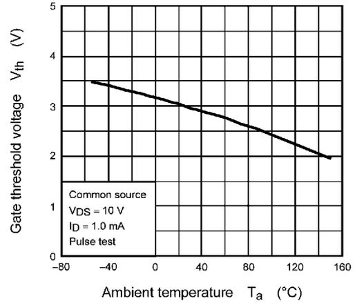
**Fig. 8.8**  $V_{th} - T_a$
