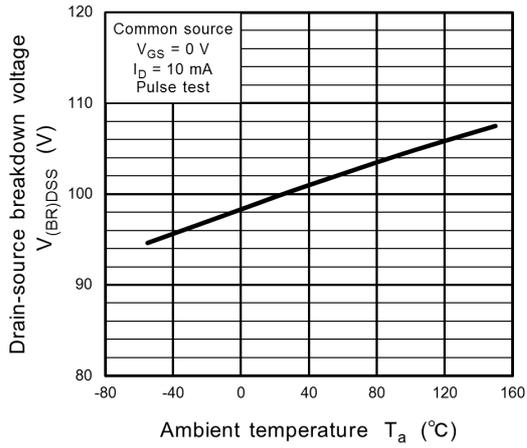
**Fig. 8.7**  $V_{(BR)DSS} - T_a$
