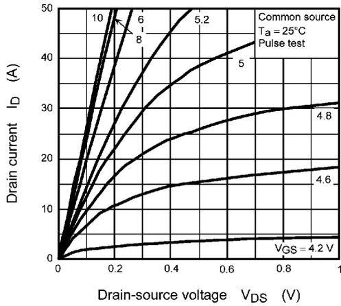
Fig. 8.1  $I_D - V_{DS}$
