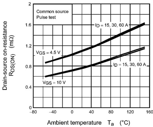
Fig. 8.9  $R_{DS(ON)} - T_a$
