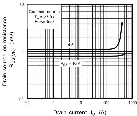
**Fig. 8.5**  $R_{DS(ON)} - I_D$
