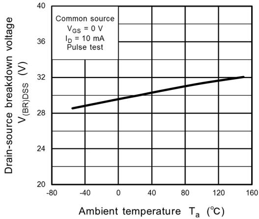
Fig. 8.7  $V_{(BR)DSS} - T_a$
