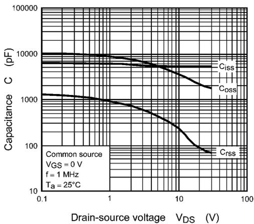
Fig. 8.11 Capacitance -  $V_{DS}$
