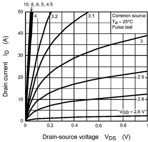
**Fig. 8.1**  $I_D - V_{DS}$
