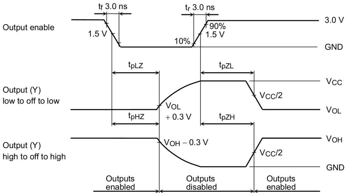
Fig. 11.9.2  $t_{pLZ}$ ,  $t_{pHZ}$ ,  $t_{pZL}$ ,  $t_{pZH}$
