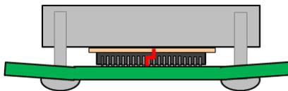
Figure 10 Substrate bending
