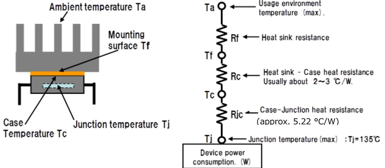
**Figure 11 Selecting a heat sink**
