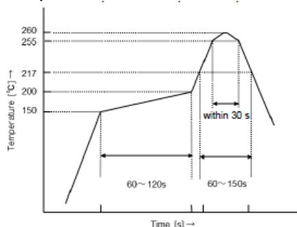
Figure 7 Typical package temperature profile
