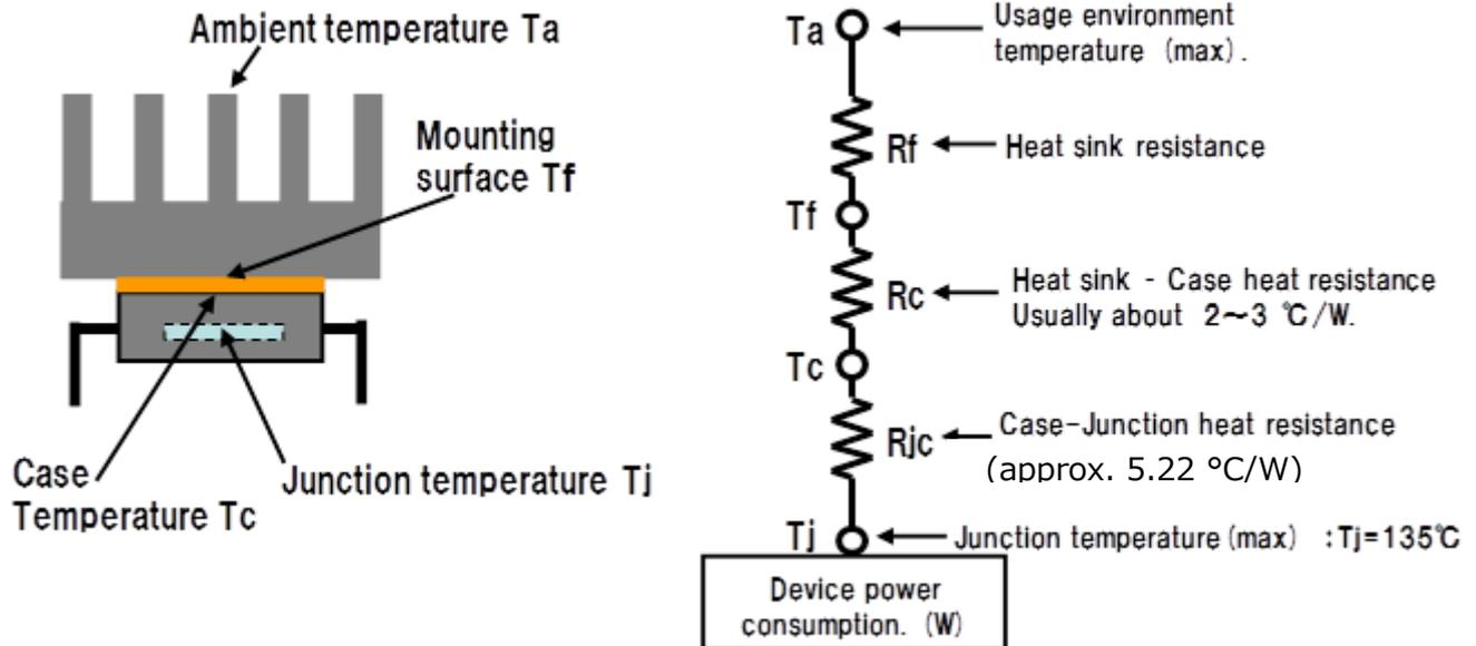
**Figure 11 Selecting a heat sink**
