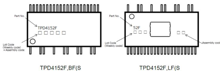
Figure 2 HSSOP31 package typical markings
