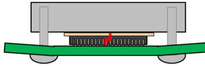
**Figure 10 Substrate bending**
