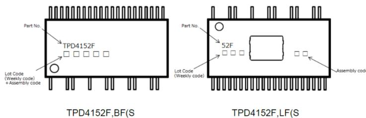
Figure 2 HSSOP31 package typical markings
