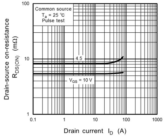
**Fig. 8.8  $R_{DS(ON)} - I_D$**
