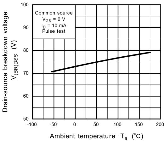
**Fig. 8.11  $V_{(BR)DSS} - T_a$**
