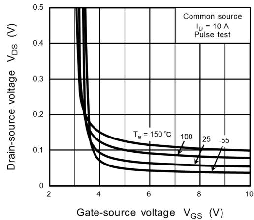
**Fig. 8.4  $V_{DS} - V_{GS}$**
