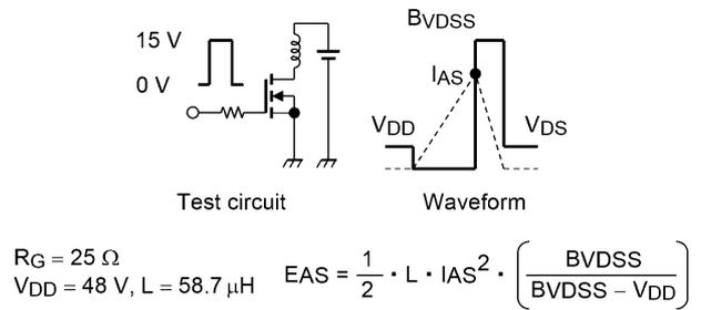
**Fig. 8.16 Test Circuit/Waveform**
