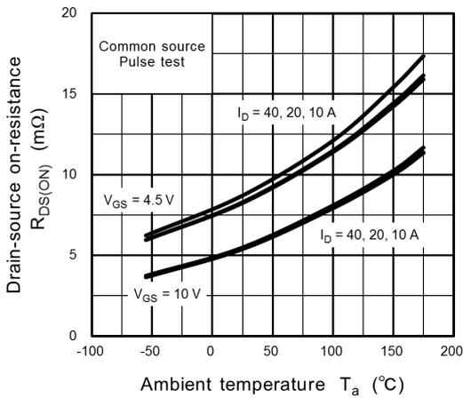
**Fig. 8.9  $R_{DS(ON)} - T_a$**
