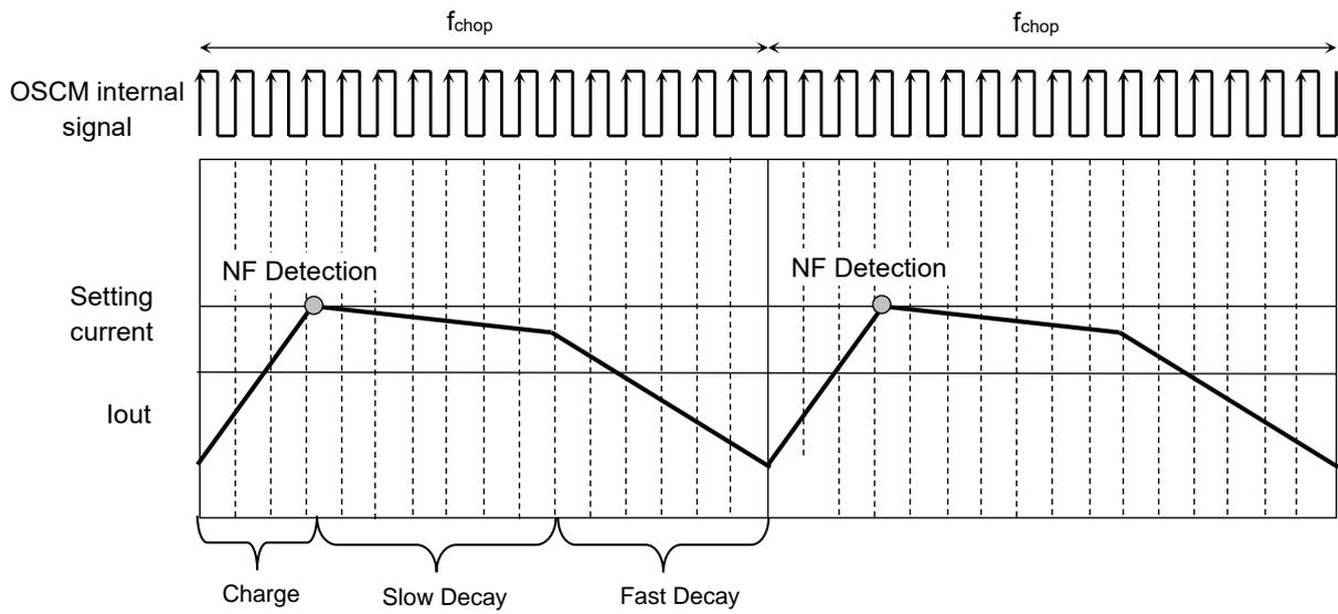
**Figure 9.1.5.1 Mixed Decay Waveform (Current Waveform) \*Charge → Slow Decay → Fast Decay**
