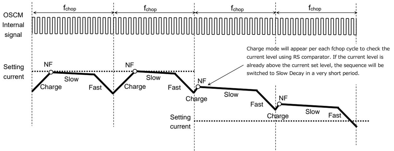
**Figure 9.1.5.3.3 When the Next Current Step is lower**
