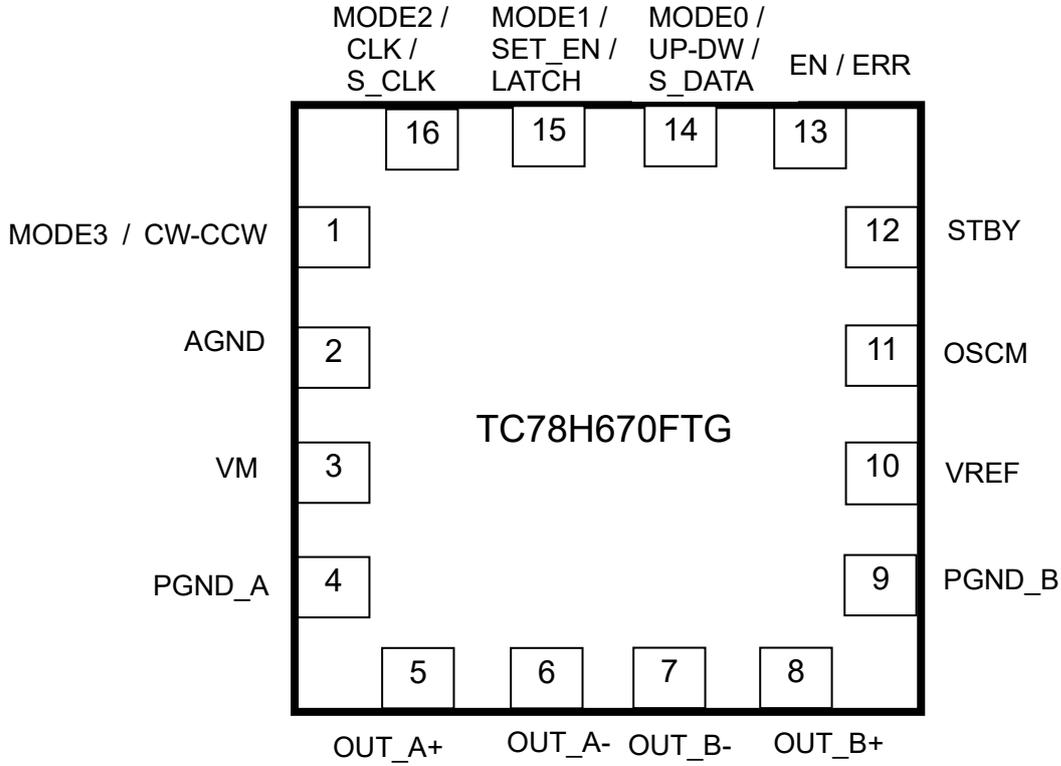
**Figure3 Pin Assignment**
