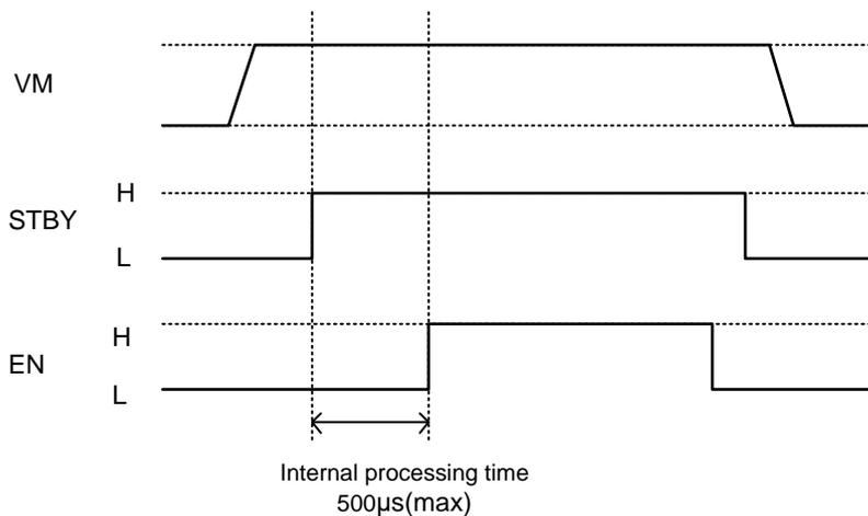
**Figure 8.2 ENABLE Function**
