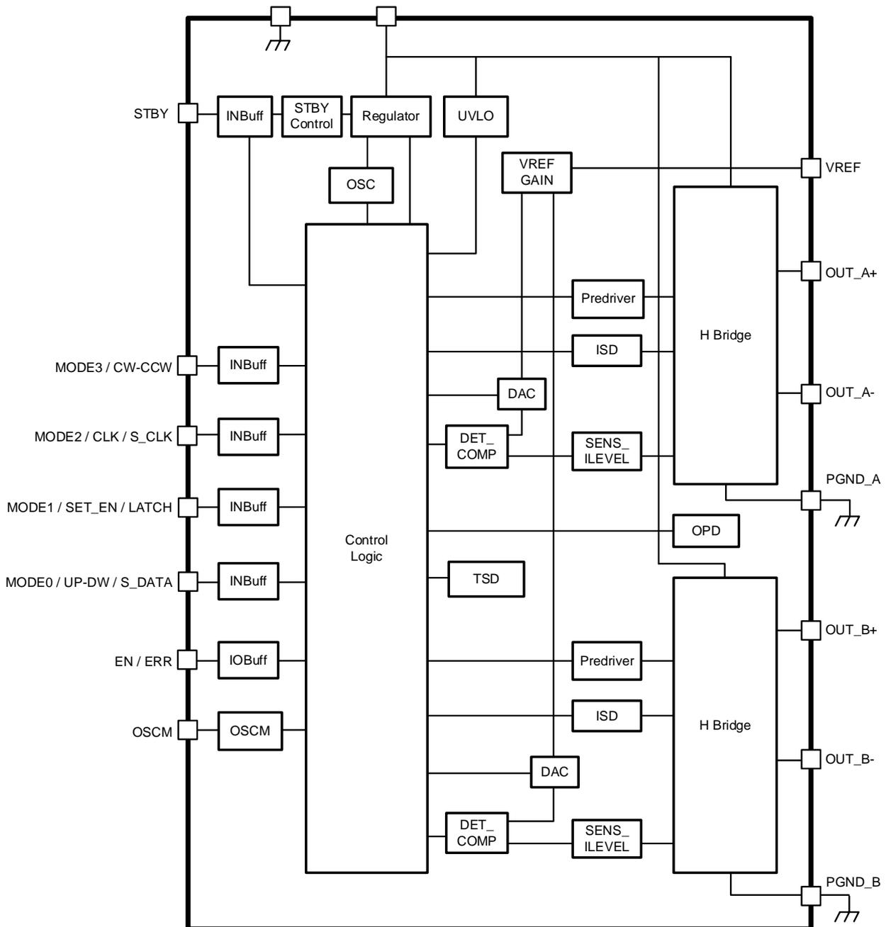
**Figure 5 Block diagram**
