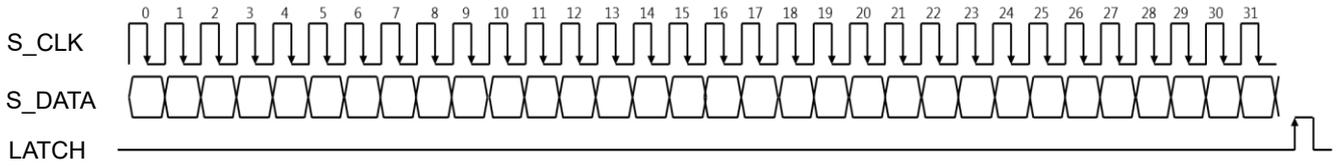
**Figure 9 When the interface is in serial mode**
