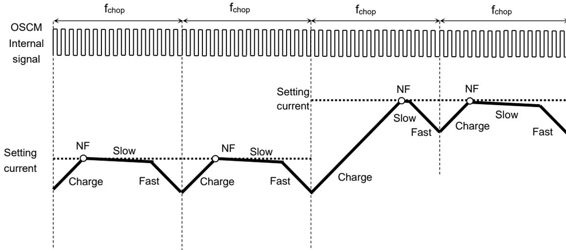
Figure 9.1.5.3.1 When the next current step is higher
