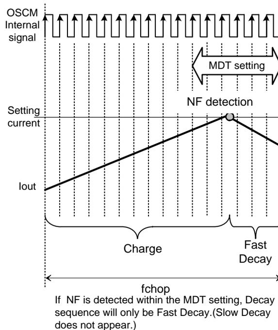
**Figure 9.1.5.2.2 If the NF detection was within the timing set by the MDT register**
