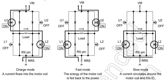
**Operation Function of Output Transistor**
