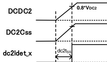
Fig.7.2 Soft start time for DCDC2
