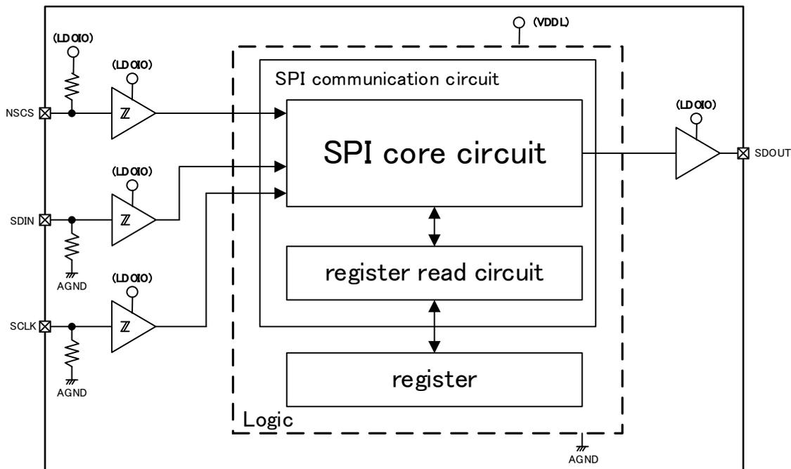
Fig. 5.7.a Block diagram for SPI communication circuit
