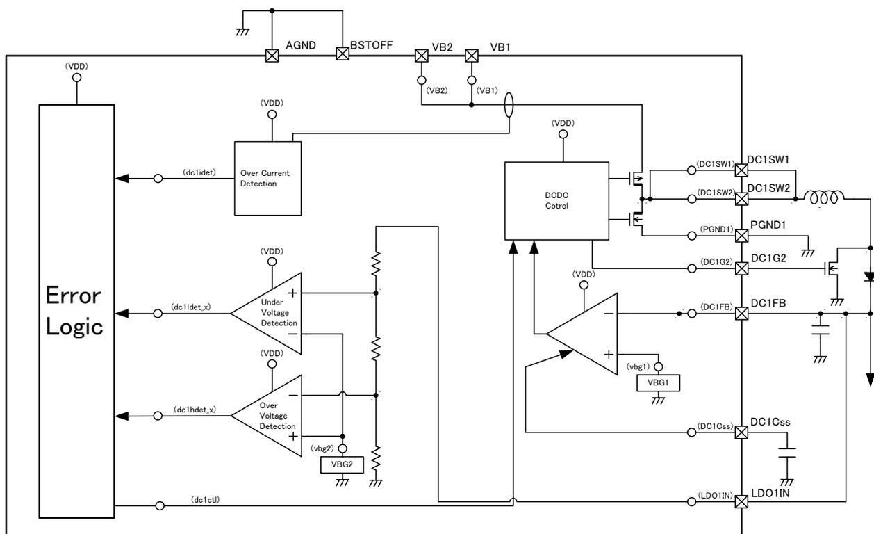
At the time of using DCDC convertor for buck mode
