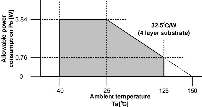
Substrate size 76.2x114.3x1.6 mm Soldering on substrate board: applicable
