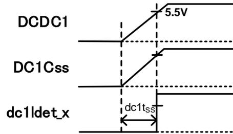
Fig.7.1 Soft start time for DCDC1
