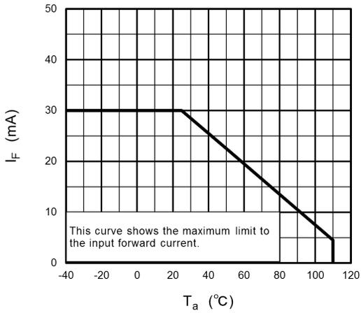
Fig. 12.1.1 I<sub>F</sub> - T<sub>a</sub>
