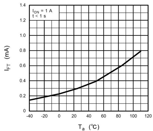
Fig. 12.1.6 I<sub>FT</sub> - T<sub>a</sub>
