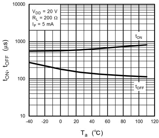
**Fig. 12.1.7  $t_{ON}, t_{OFF} - T_a$**
