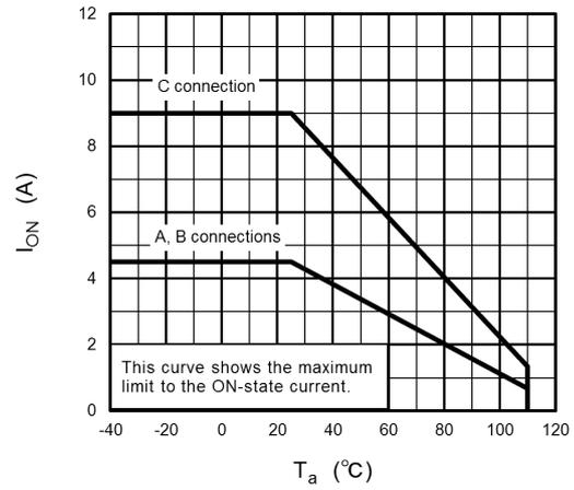
Fig. 12.1.2 I<sub>ON</sub> - T<sub>a</sub>
