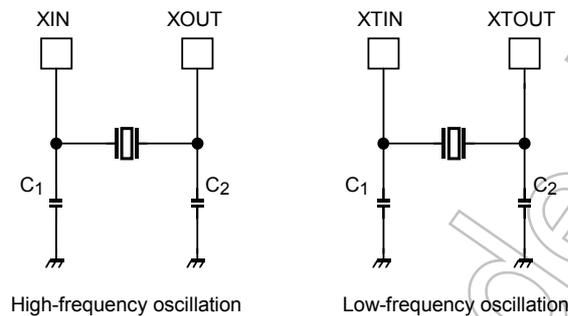
Note 1: To ensure stable oscillation, the resonator position, load capacitance, etc. must be appropriate. Because these factors are greatly affected by board patterns, please be sure to evaluate operation on the board on which the device will actually be mounted.
