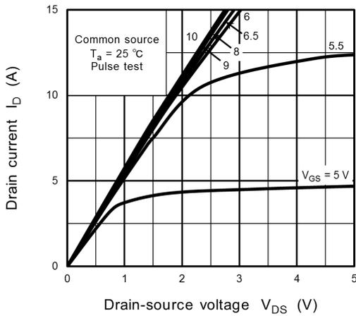
Fig. 8.1  $I_D - V_{DS}$
