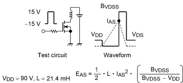
**Fig. 8.16 Test Circuit/Waveform**
