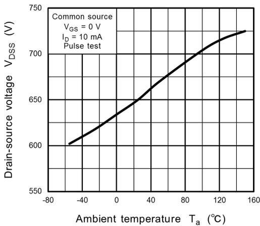
Fig. 8.5  $V_{DSS} - T_a$
