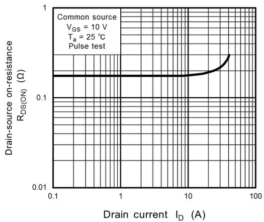
Fig. 8.6  $R_{DS(ON)} - I_D$
