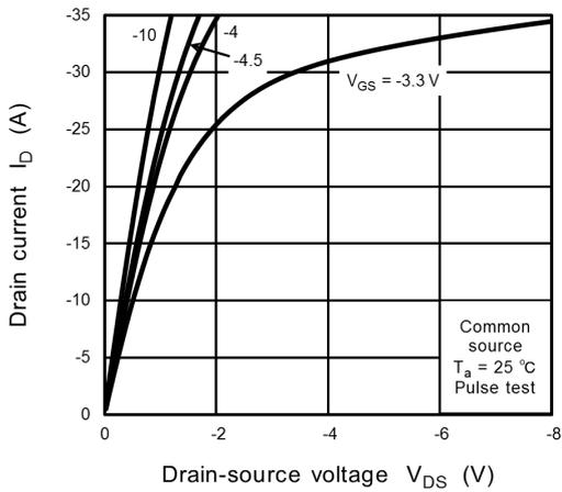
Fig. 8.1  $I_D - V_{DS}$
