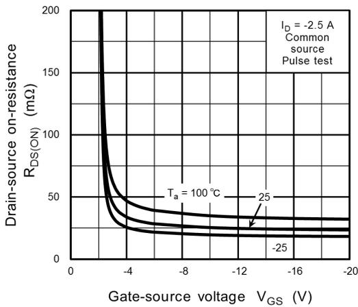
Fig. 8.3  $R_{DS(ON)} - V_{GS}$
