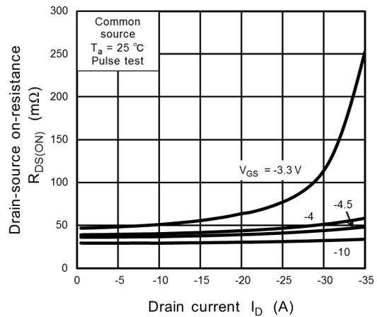
Fig. 8.4  $R_{DS(ON)} - I_D$
