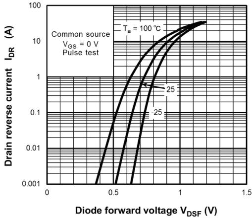
Fig. 8.7  $I_{DR} - V_{DSF}$
