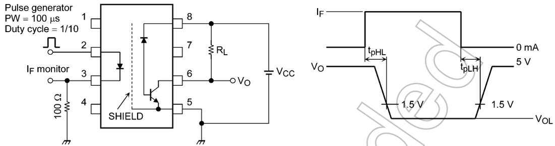
Fig. 12.1.1 Switching Time Test Circuit and Waveform
