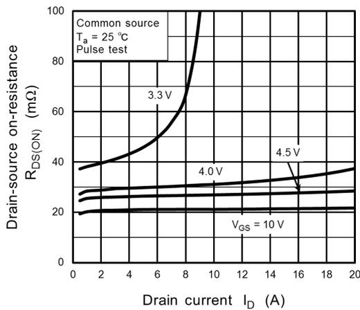
**Fig. 8.5  $R_{DS(ON)} - I_D$**
