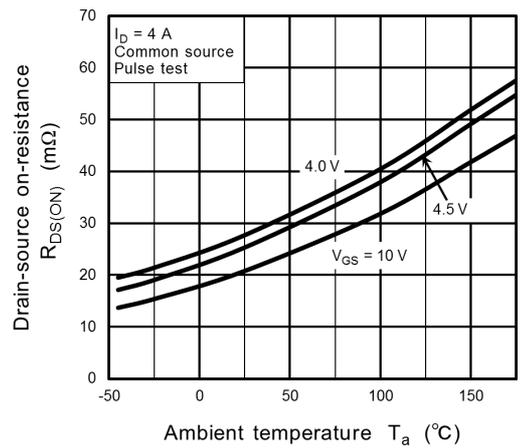
**Fig. 8.6  $R_{DS(ON)} - T_a$**
