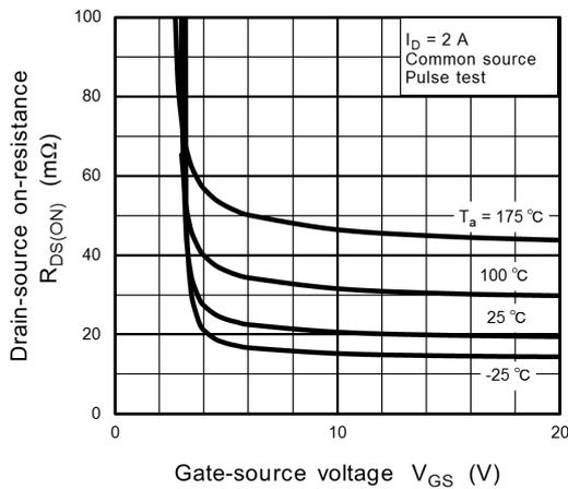
**Fig. 8.3  $R_{DS(ON)} - V_{GS}$**
