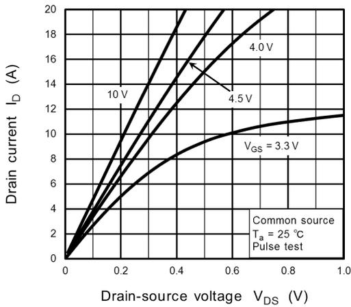
**Fig. 8.1  $I_D - V_{DS}$**
