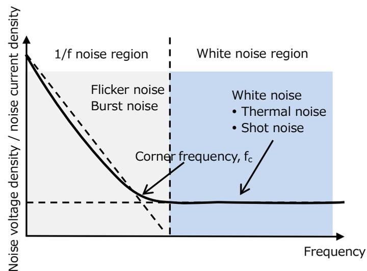
**Figure 3.1.3 Frequency characteristics of op amp circuit noise**
