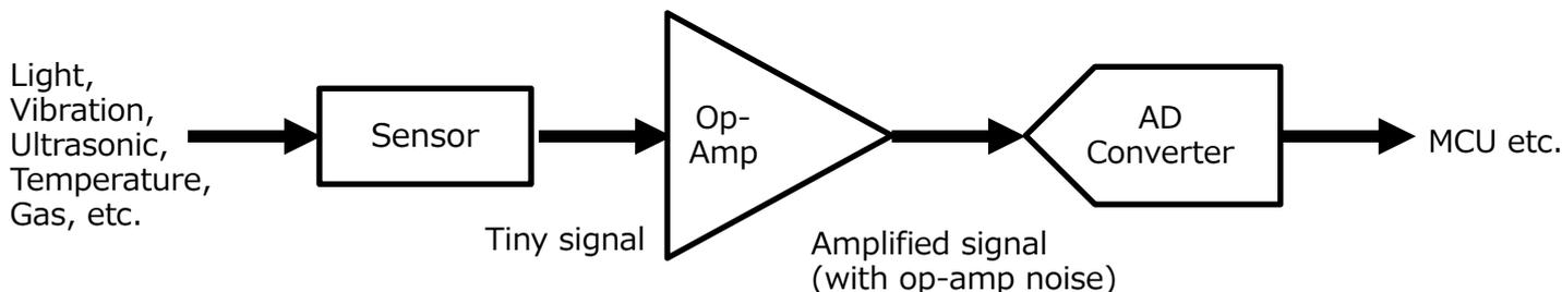
**Figure 2.1 Example of a sensor circuit block**
