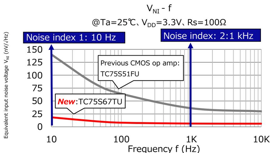
The equivalent input noise voltage of the TC75S67TU is roughly 86% lower at 10 Hz and roughly 82% lower at 1 kHz than that of Toshiba’s previous CMOS op amp.
