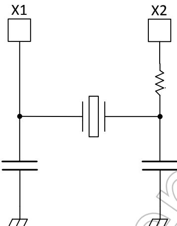
**Figure 7.7 Oscillation circuit sample**
