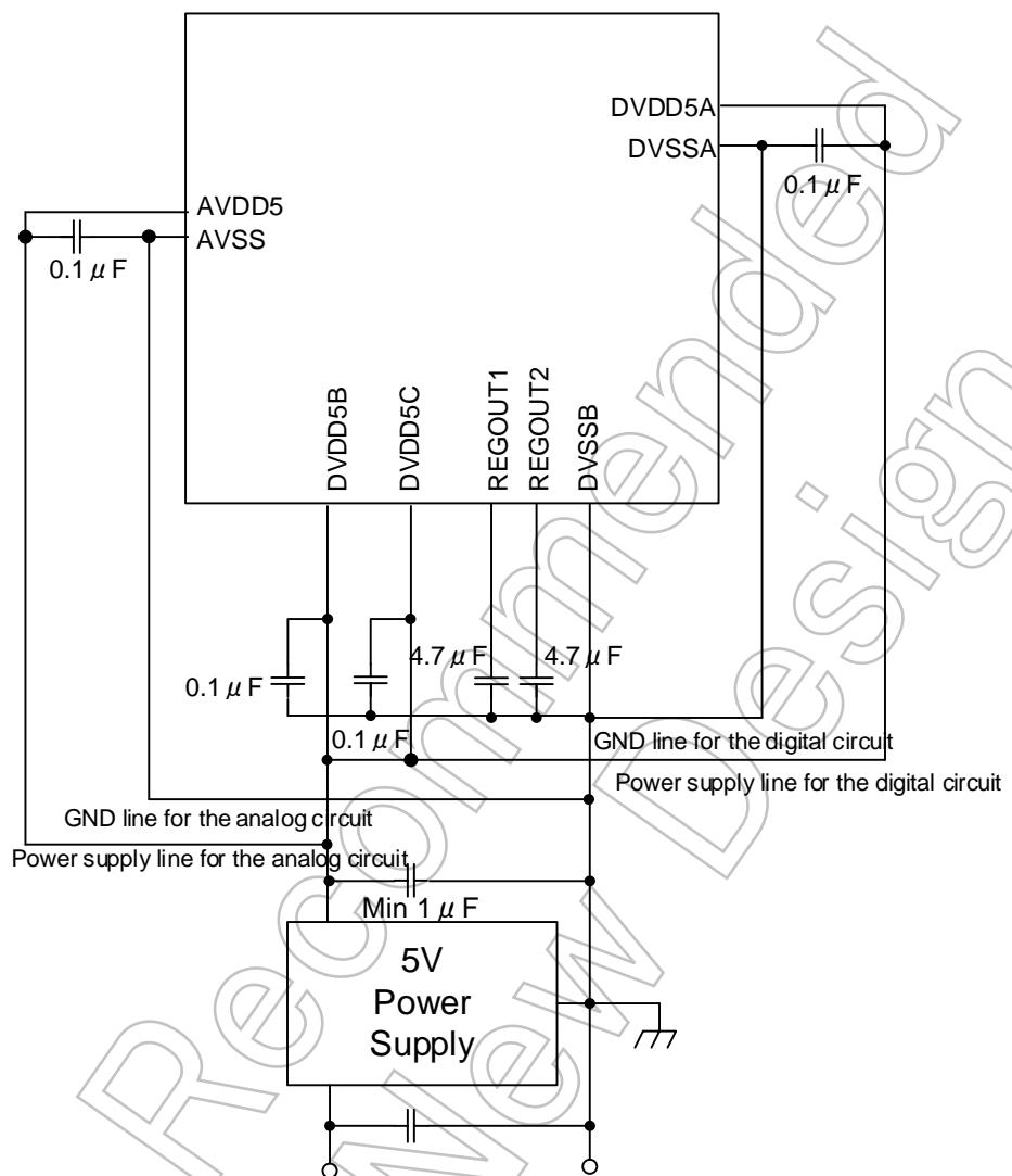
**Figure 4.1 Capacitors for power supply pins connection circuit**
