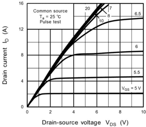
Fig. 8.1  $I_D - V_{DS}$
