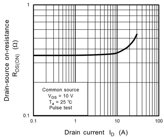
Fig. 8.6  $R_{DS(ON)} - I_D$
