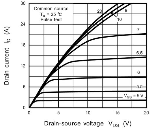
Fig. 8.2  $I_D - V_{DS}$
