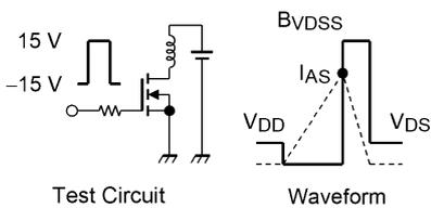
$V_{DD} = 90 \text{ V}, L = 4.77 \text{ mH}$
