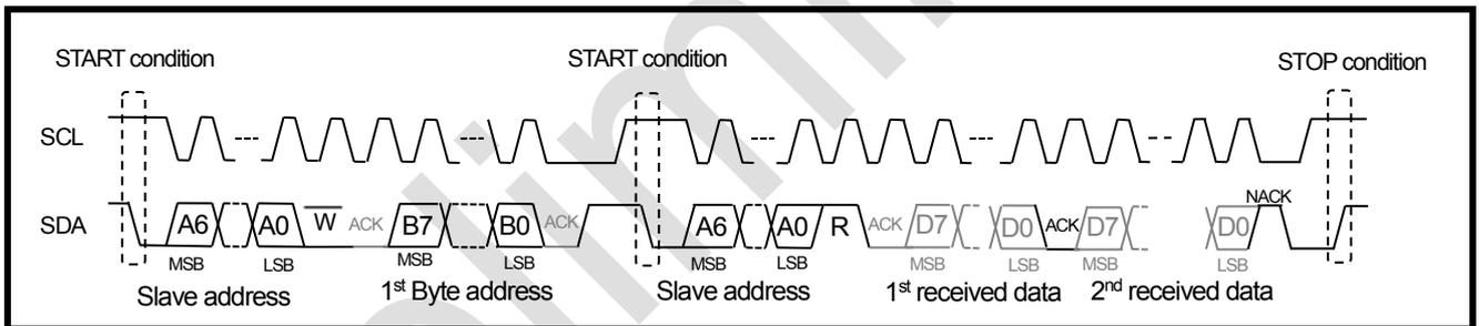
**Figure 4-15 I<sup>2</sup>C transfer format (read 2-byte data from serial memory)**
