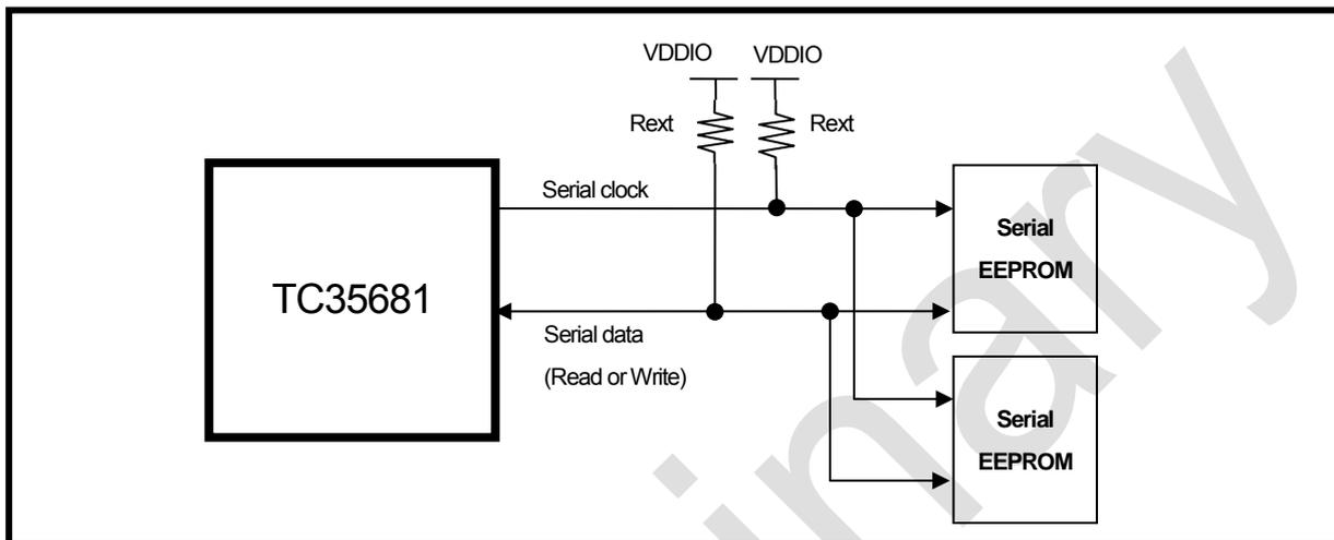
**Figure 4-13 Example of the connection with serial EEPROM's through I<sup>2</sup>C interface (open-drain output mode)**
