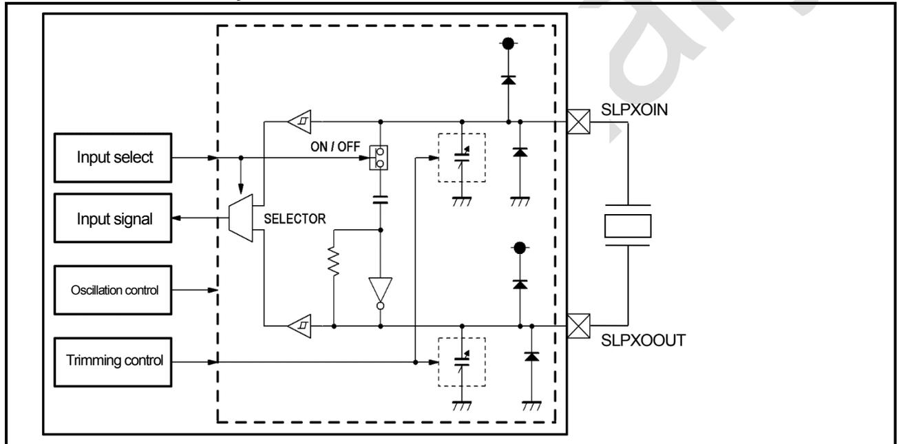
Figure 4-21 Connection of Crystal resonator
