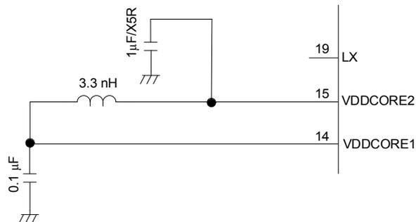
Figure 6-3 Circuit for LDO regulator
