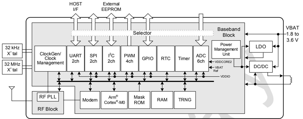
Figure 3-1 Internal block diagram of TC35681 and an example of connection of main components
