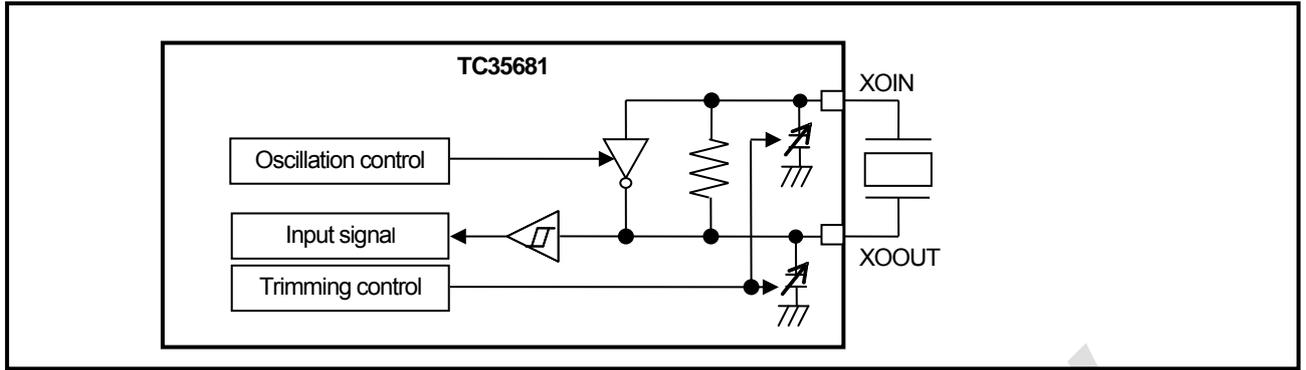
Figure 4-20 Connection of a crystal resonator
