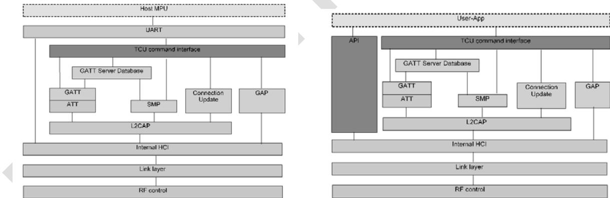
Figure 3-3 Example of system configuration of TC35681
