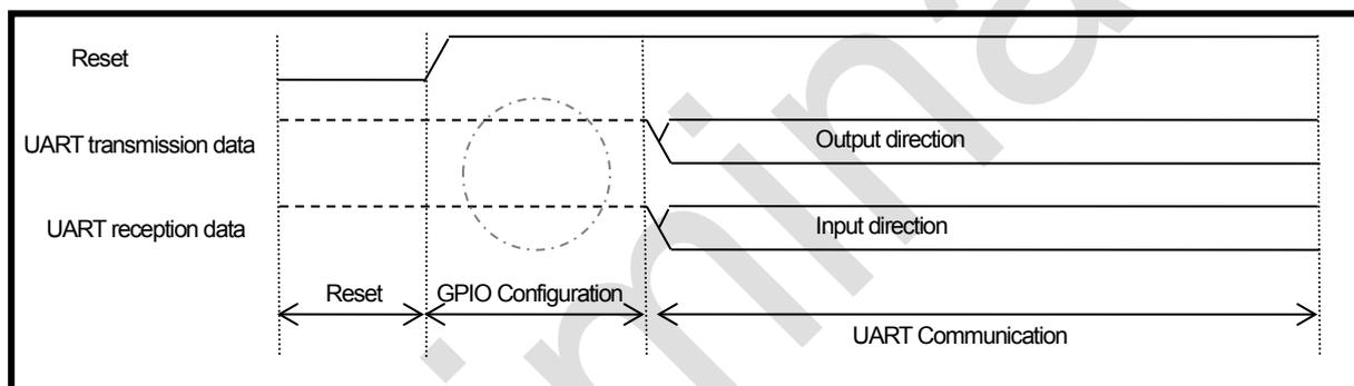
**Figure 4-4 Timing of assignment of UART function**
