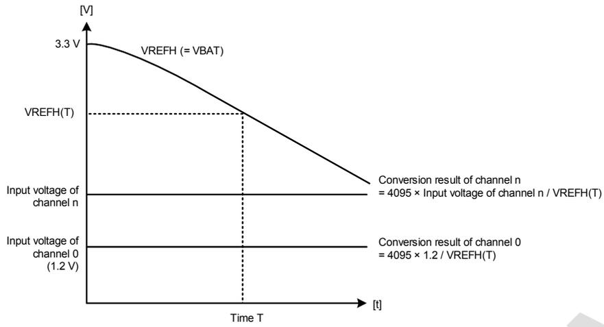
Figure 4-19 Conceptual diagram of the voltage conversion
