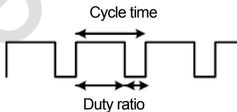
Figure 4-17 PWM pulse waveform
