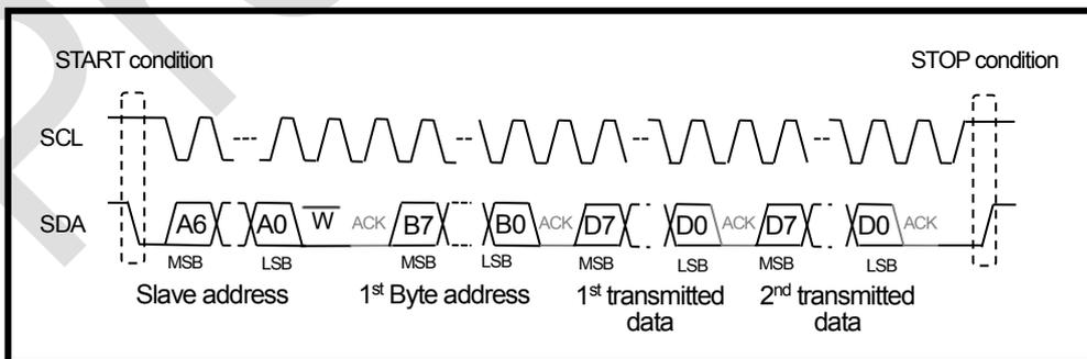
**Figure 4-16 I<sup>2</sup>C transfer format (write 2-byte data to serial memory write)**
