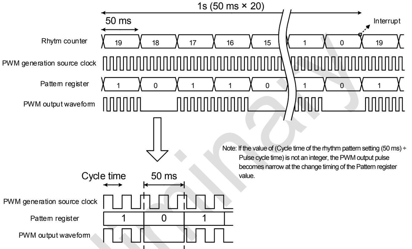
Figure 4-18 Output masking by PWM rhythm function
