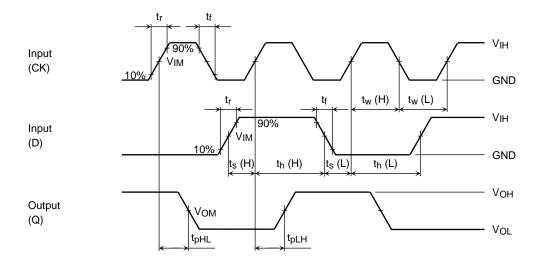
Figure 2 t<sub>pLH</sub>, t<sub>pHL</sub>, t<sub>w</sub>, t<sub>s</sub>, t<sub>h</sub>
