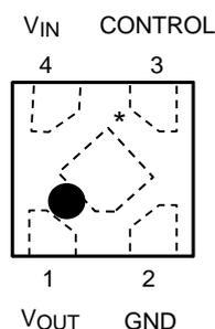
\*Center electrode should be connected to GND or Open
