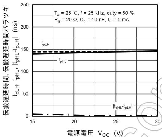
図 13.2.15  $t_{pLH}, t_{pHL}, |t_{pHL} - t_{pLH}| - V_{CC}$
