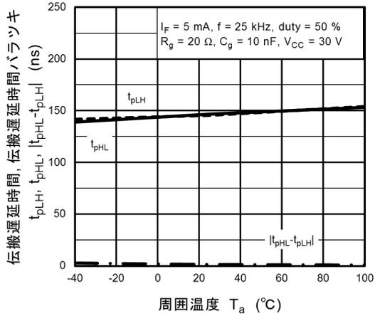
図 13.2.13  $t_{pLH}, t_{pHL}, |t_{pHL} - t_{pLH}| - T_a$
