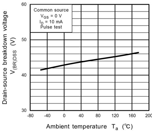
**Fig. 8.11  $V_{(BR)DSS} - T_a$**
