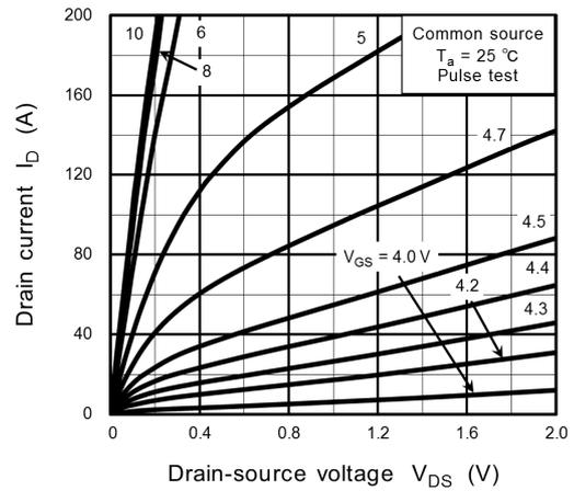
Fig. 8.2  $I_D - V_{DS}$
