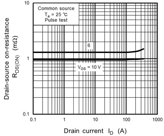
**Fig. 8.8  $R_{DS(ON)} - I_D$**
