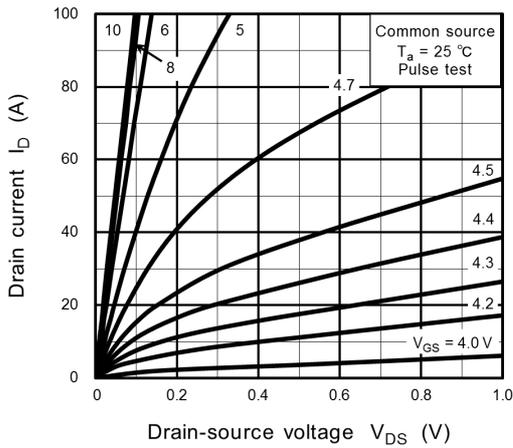
Fig. 8.1  $I_D - V_{DS}$
