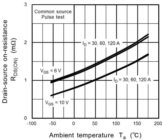
**Fig. 8.9  $R_{DS(ON)} - T_a$**
