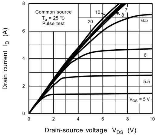
**Fig. 8.1**  $I_D - V_{DS}$
