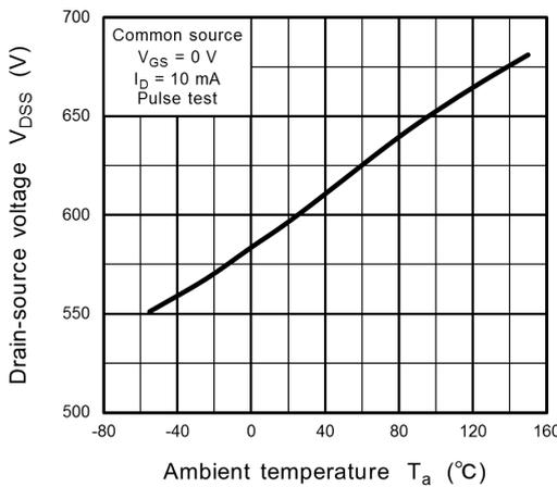
**Fig. 8.5**  $V_{DSS} - T_a$
