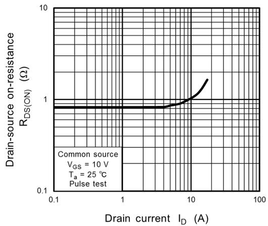
**Fig. 8.6**  $R_{DS(ON)} - I_D$
