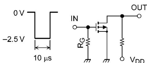
Fig. 6.3.1 Test Circuit of Switching Time
