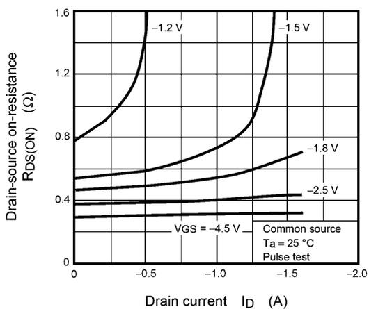
**Fig. 8.5  $R_{DS(ON)} - I_D$**
