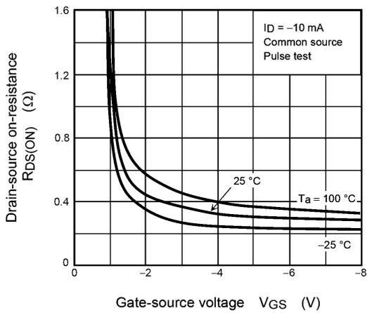
**Fig. 8.3  $R_{DS(ON)} - V_{GS}$**
