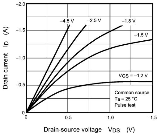
**Fig. 8.1  $I_D - V_{DS}$**
