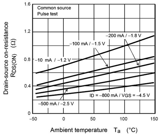
**Fig. 8.6  $R_{DS(ON)} - T_a$**
