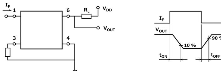
Fig. 11.1 Switching Time Test Circuit and Waveform
